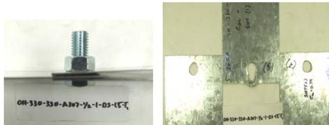
Figure 7 Failure mode of double shear connection OH-330-330-A307-1/2-1-DS-1.5-T1
