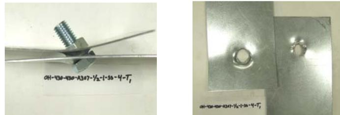
**Figure 9 Failure mode of single shear connection OH-430-430-A307-1/2-1-SS-4-T1**
