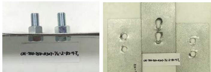
Figure 12 Failure mode of double shear connection OH-300-300-A307-1/2-1-DS-4-T1
