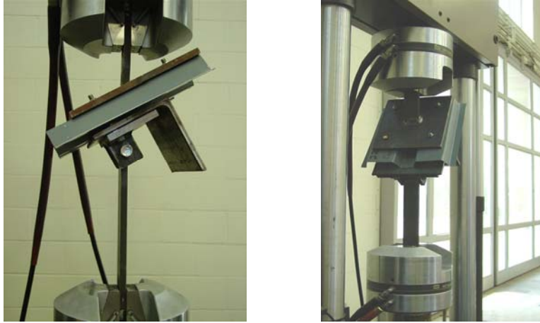
Figure 6. Test Specimen Mounted in the Test Fixture
