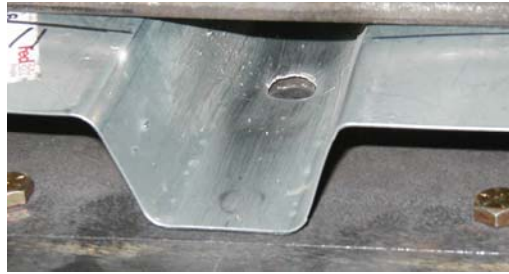
Figure 7. Typical Failed Test Specimen
