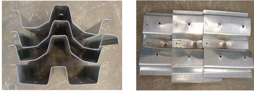
Figure 8. Deformation of Deck Type B3 and B4
