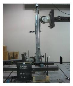
Figure 5 – Raised hold-down Assembly Tension Test Setup – Side
