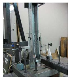
Figure 6 – Raised hold-down Assembly Tension Test Setup – Front
