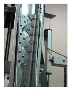
Figure 7 - Hold-down Assembly Tension Test Failure – Screw Shear
