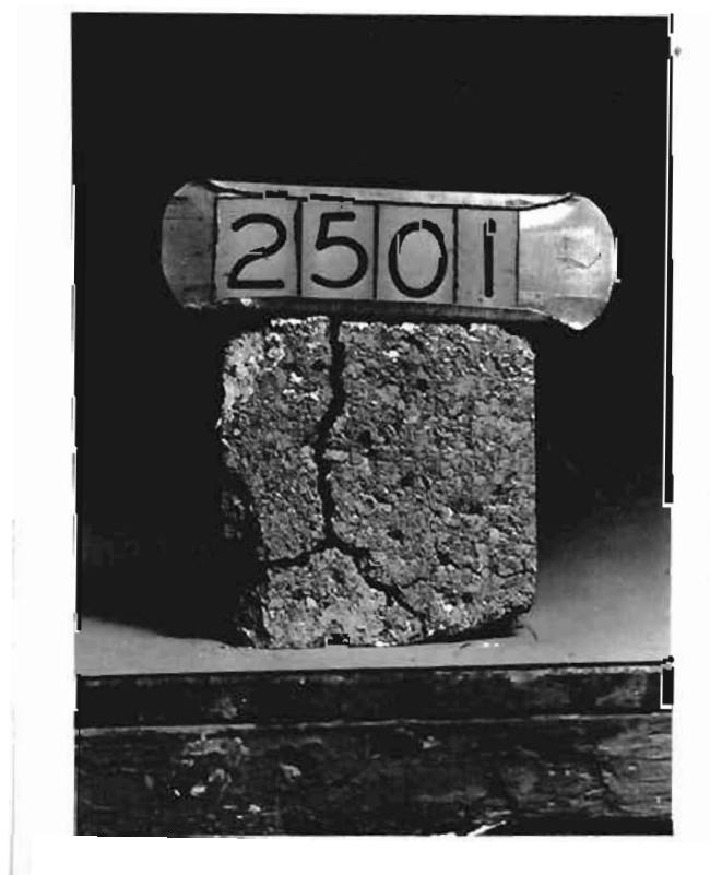
Fig. 25 - Resistance to CO of Regular Burn, Super Duty, Missouri fire brick
