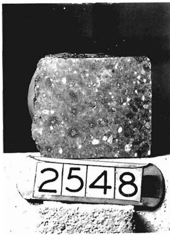
Fig. 49 - Polished Section of "C" ( 4\frac{1}{2} x 9 x 18") After Reheat - 2X
