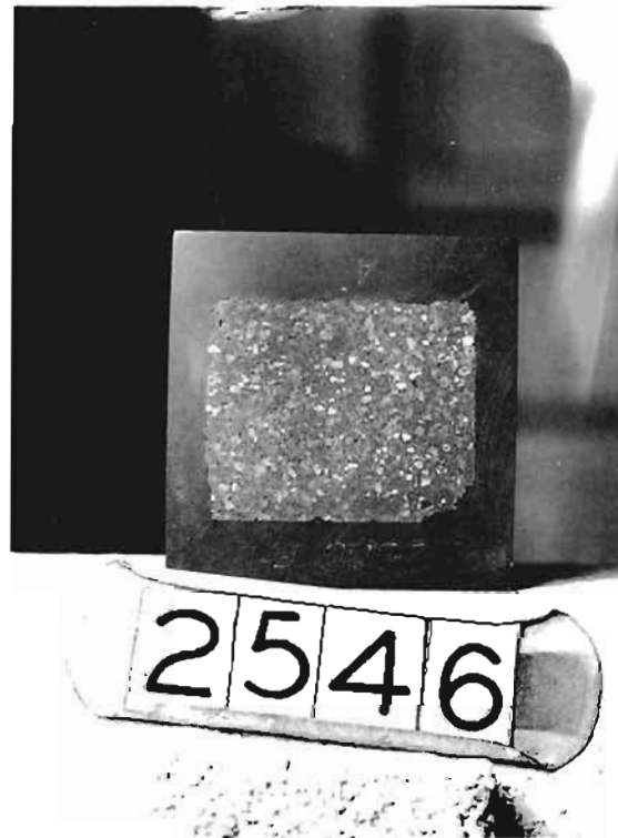
Fig. 47 - Polished Section of "A" ( 4\frac{1}{2} x 9 x 18") After Reheat - 2X
