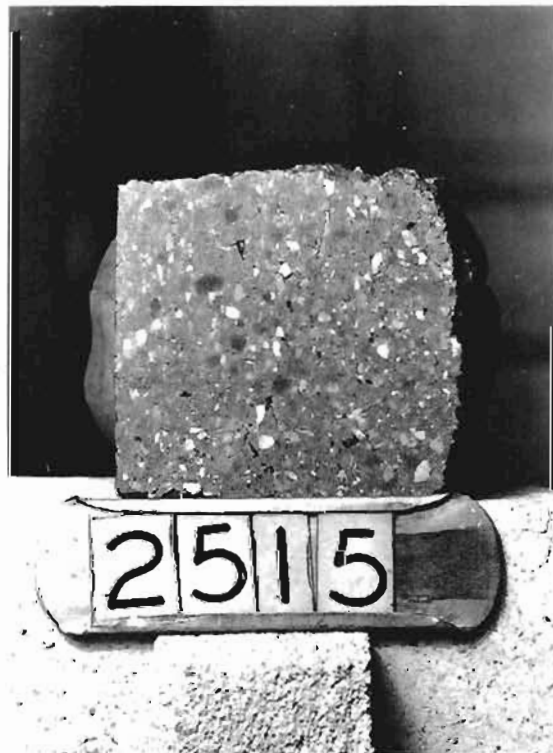
Fig. 29 - Polished Section of Hard Burned, Super Duty, Missouri fire brick ( 4\frac{1}{2} x 9 x 18") Before Reheat 2X
