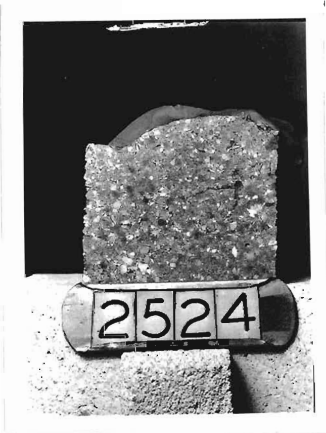
Fig. 37 - Polished Section of Super Duty Missouri fire brick ( 4\frac{1}{2} x 9 x 18") After Reheat 2X
