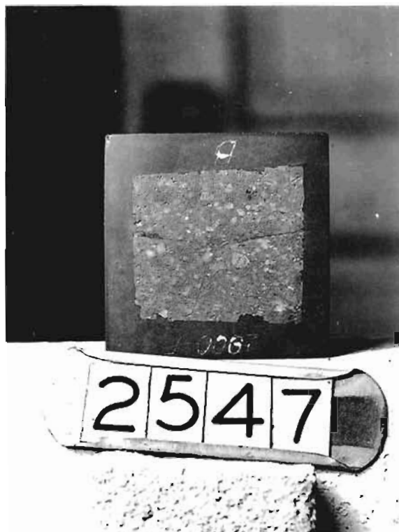
Fig. 48 - Polished Section of "B" ( 4\frac{1}{2} x 9 x 18") After Re- heat - 2X
