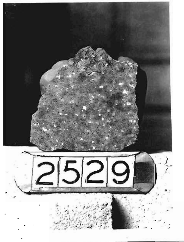
Fig. 41 - Polished Section of "B" Hearth & Bosh Quality fire brick After Reheat 2X
