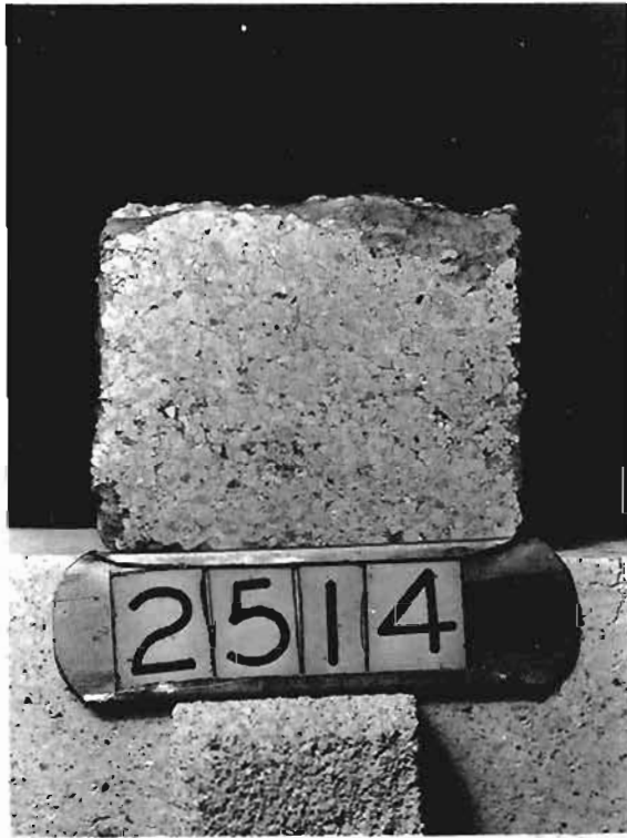
Fig. 28 - Polished Section of Super Duty Missouri fire brick ( 4\frac{1}{2} x 9 x 18") Before Reheat 2X
