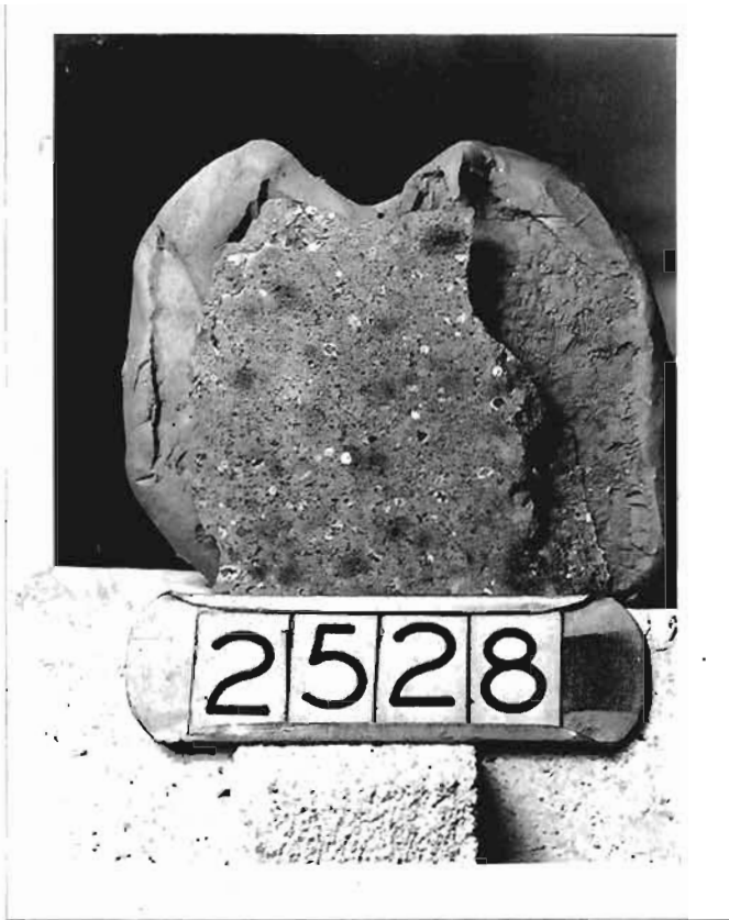
Fig. 40 - Polished Section of "A" Hearth & Bosh Quality fire brick After Re-heat - 2X
