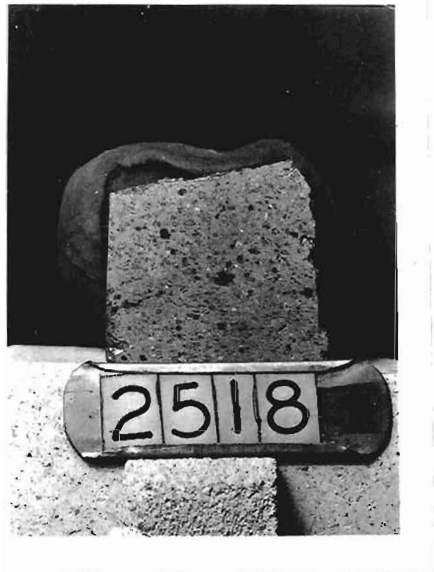
Fig. 31 - Polished Section of "A" Hearth & Bosh Quality fire brick Before Re- heat - 2X
