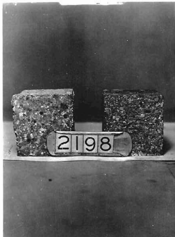
Fig. 21 - Resistance to CO of Hard Burned, Super Duty, Missouri fire brick.
