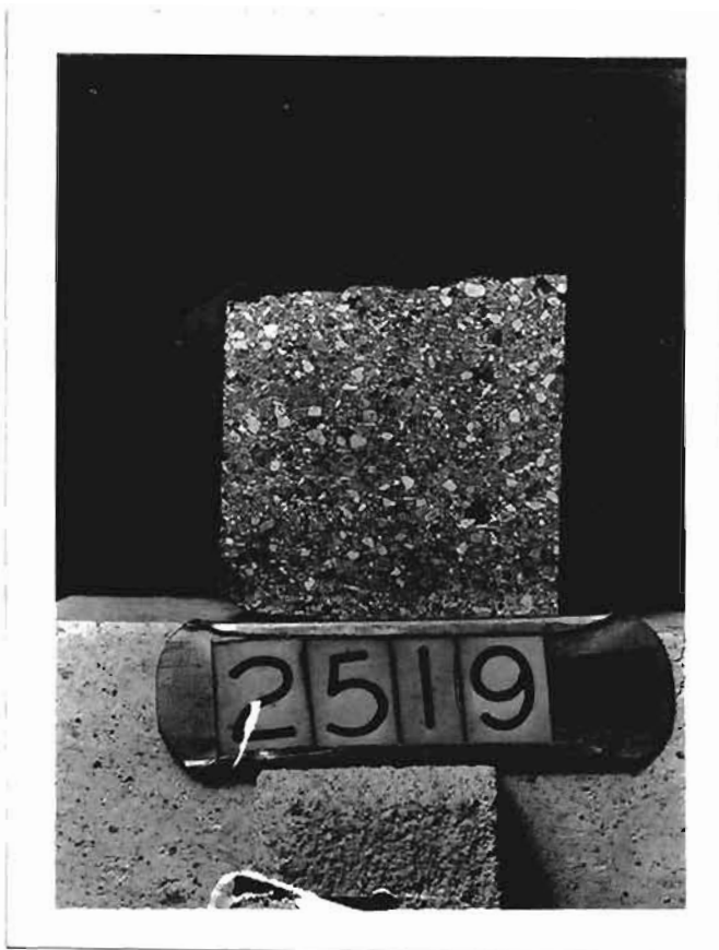
Fig. 32 - Polished Section of "B" Hearth & Bosh Quality fire brick Before Re- heat - 2X
