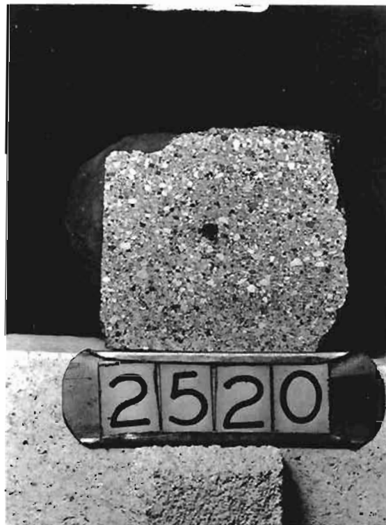
Fig. 33 - Polished Section of "B" Inwall Quality fire brick Before Reheat - 2X
