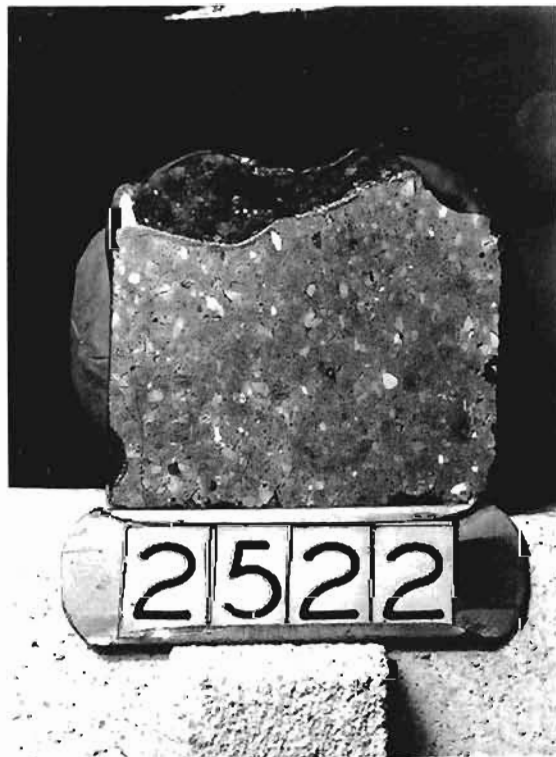
Fig. 35 - Polished Section of Missouri Super Duty Inwall Quality fire brick After Reheat 2X
