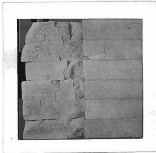
Fig. 15 Column of Standard Top Quality Blast Furnace Refractory at the left shows a 9% loss after being subjected to spalling test. The Hard Burned Super Duty material at the right subjected to the same spalling test shows a loss of only three tenths of one per cent.
