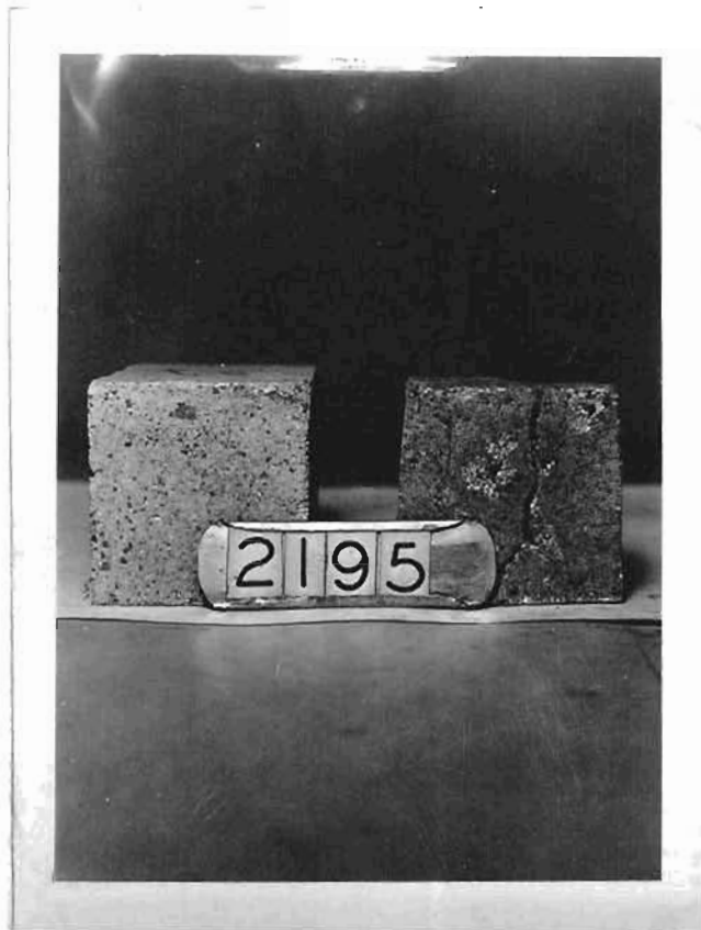
Fig. 19 - Resistance to CO of "B" Inwall Quality
