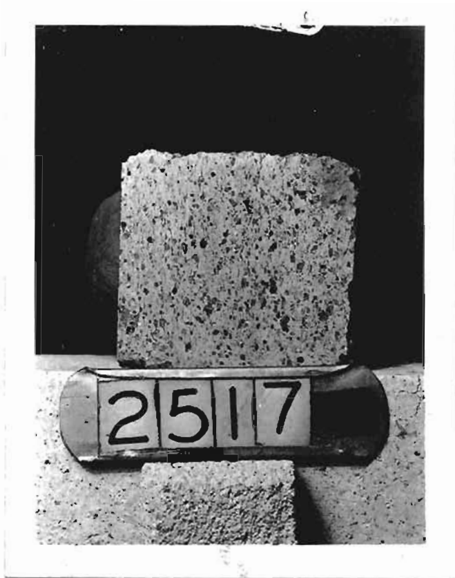
Fig. 30 - Polished Section of "A" Inwall Quality fire brick Before Reheat - 2X
