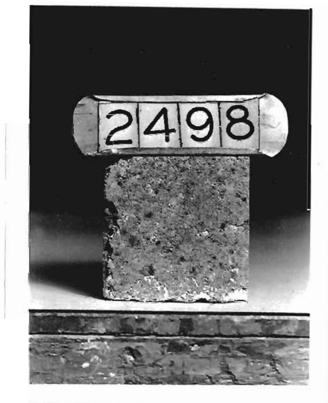
Fig. 24 - Resistance to CO of Missouri First Quality fire brick
