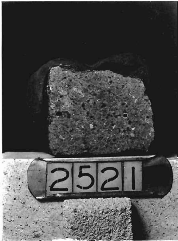
Fig. 34 - Polished Section of Missouri First Quality fire brick Before Reheat - 2X
