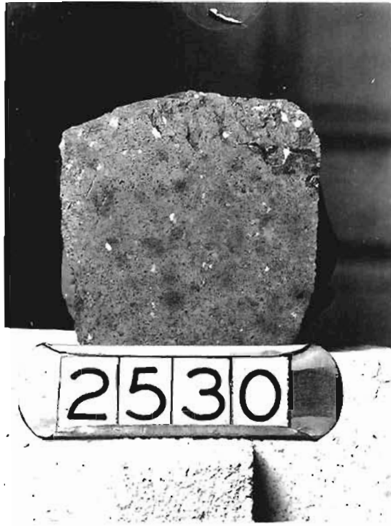
Fig. 42 - Polished Section of "B" Inwall Quality fire brick After Reheat - 2X
