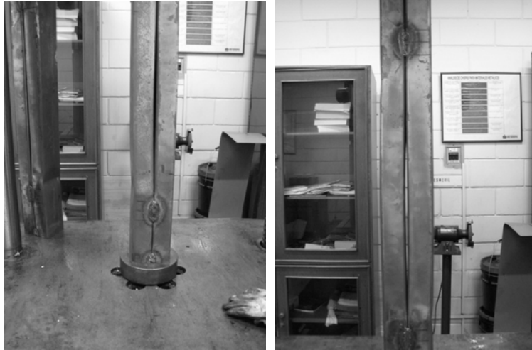
Figure 7 Other failure modes for rigidly supported specimens
