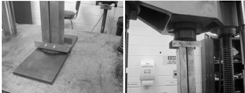
Figure 5 Test setup for the flexible support condition
