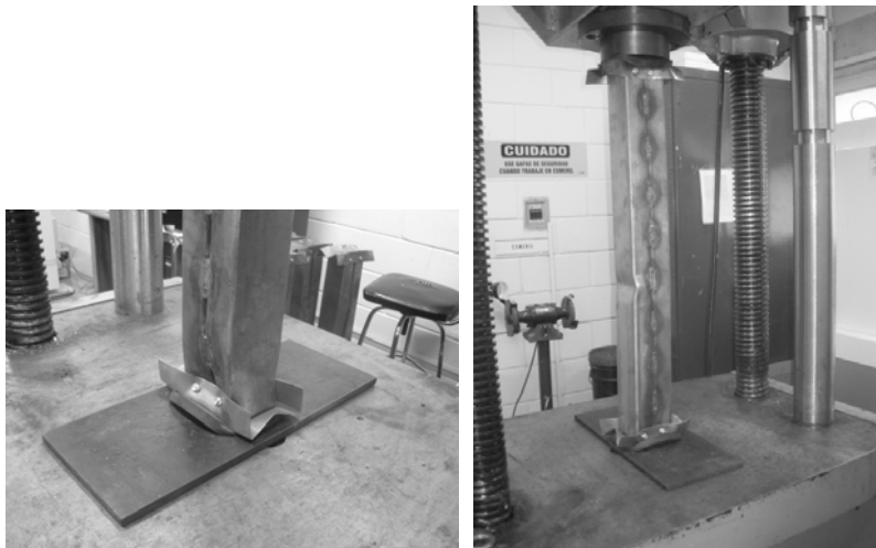
Figure 8 Local buckling at ends for samples with flexible supports (left) and buckling close to seam welds along the specimen (right).
