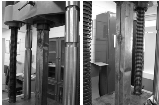
Figure 6 Typical failure mode for rigidly supported specimens
