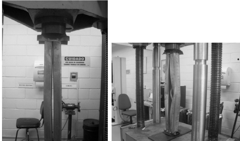
Figure 9 Failure curvature mode typical on samples with flexible supports and welds spaced 900 mm (there was a reduction in the maximum load capacity under this configuration)
