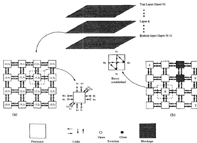
Fig. 1. A 3D RMESH with  $4 \times 4 \times N$  processors
