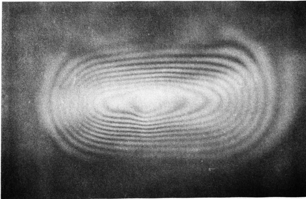
Figure VI.8. Subsidence Contours on Gelatin d=1 in., Cavity Size= 0.5 in. \times 3.5 in. \times 400 micro-in.
