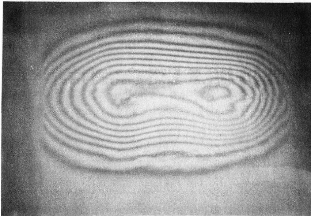
Figure VI.10. Subsidence Contours on Sand d=3 in., Cavity Size= 1 in. \times 6 in. \times 300 micro-in.
