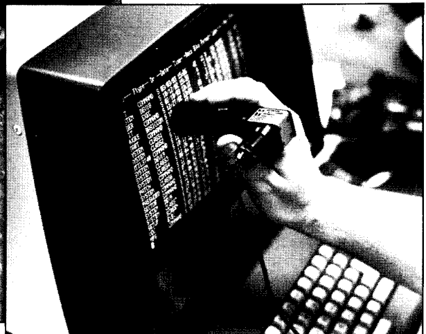
This woman is reading the screen with a product called Optacon (Optical Tactile Converter), conceived by IEEE Life Fellow John G. Linvill. As the lens module moves across the image of a character, it converts the shape of the light onto a tactile array of vibrating rods, which can be scanned by the touch of a finger.
