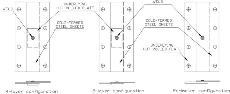
Figure 3: Steel deck panel shear test specimens
