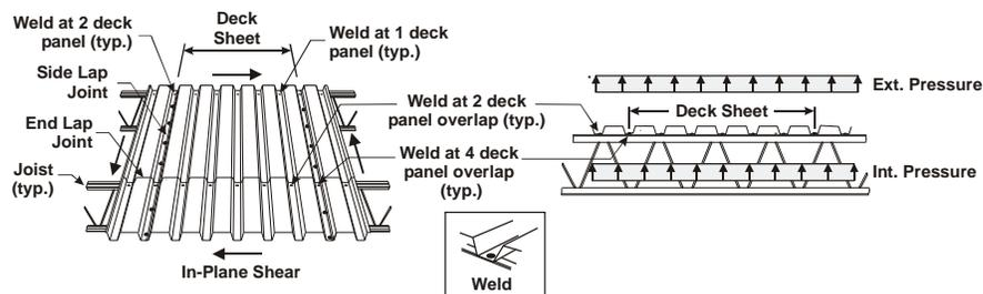
Figure 1: Steel deck panel connections and loading
