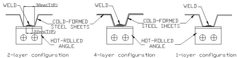
Figure 4: Steel deck panel tension test specimens
