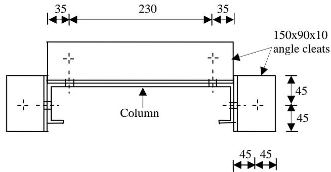
Figure (b) Plan of base connection 3
