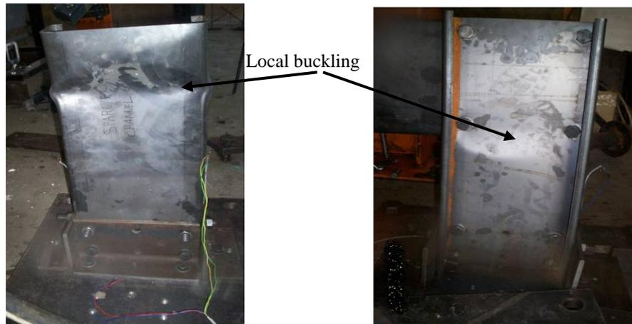
(a) Local buckling due to Load case 1      (b) Local buckling due to Load Case 4
