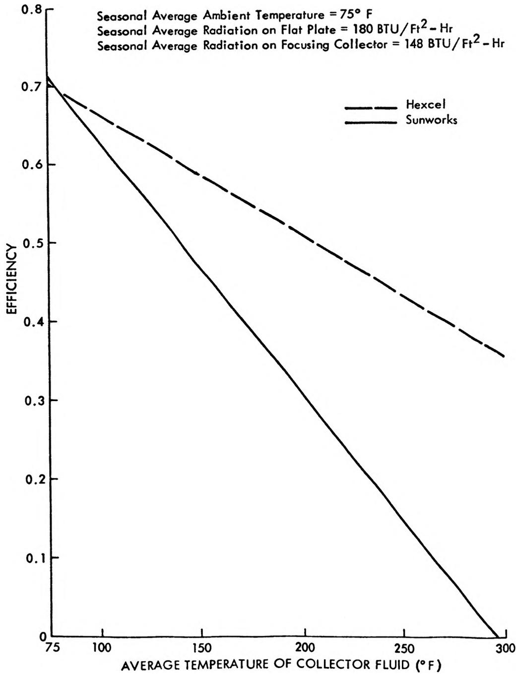
Figure 3 - Efficiency of Sunworks and Hexcel Collectors Versus Average Temperature of Collector Fluid
