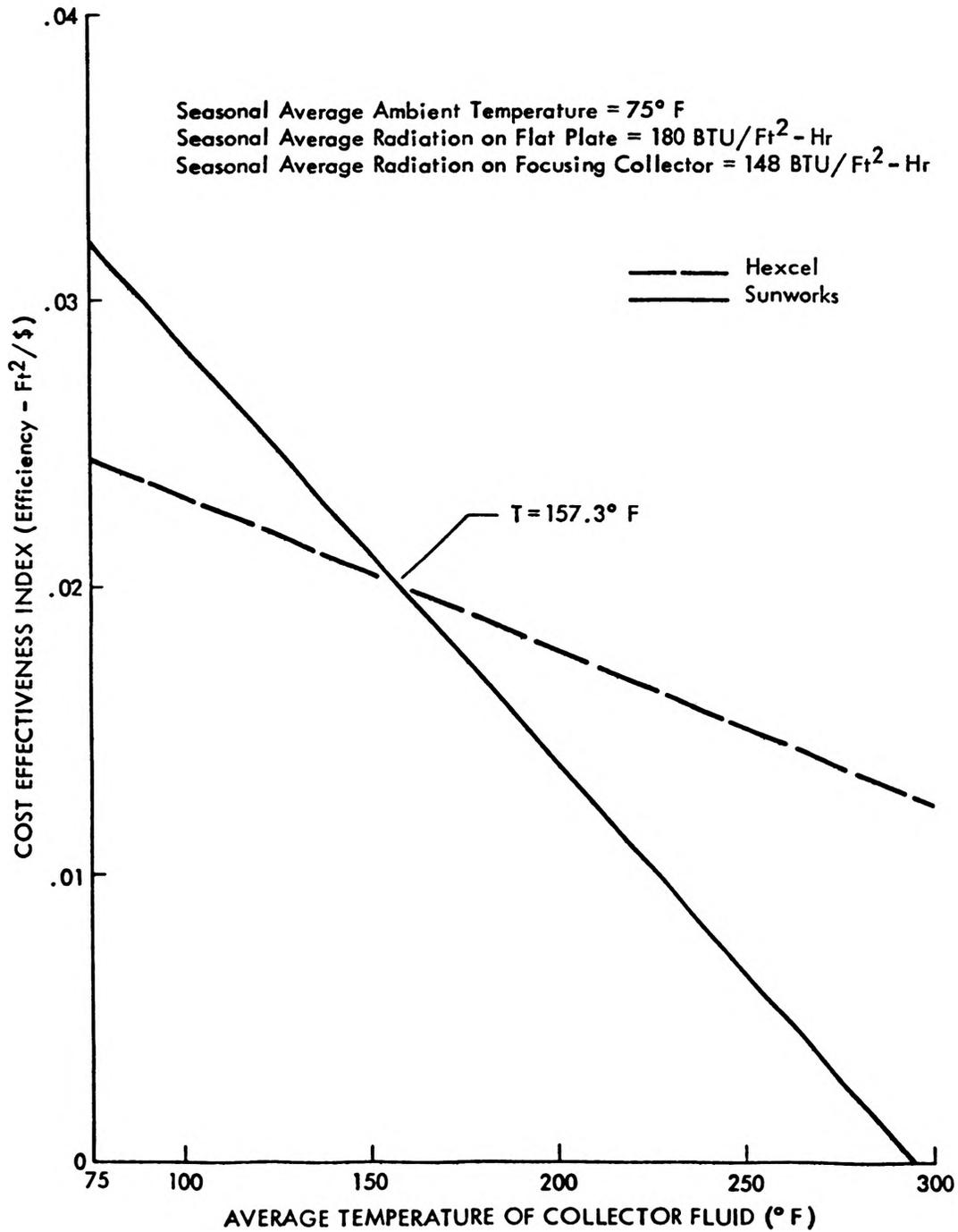
Figure 4 - Cost Effectiveness Index Versus Average Temperature of Collector Fluid for Sunworks and Hexcel Collectors
