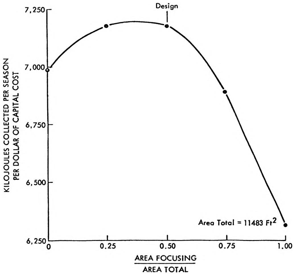
Figure 5 - Sensitivity Analysis of Energy Output Per Season Per Dollar of Capital Cost for Different Areas of Sunworks and Hexcel Collectors
