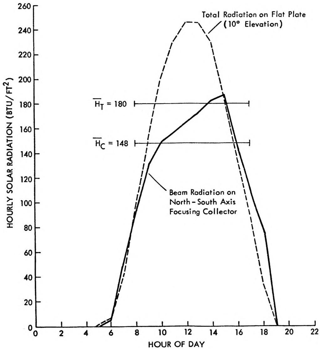
Figure 2 - Average Hourly Insolation During the Alfalfa Dehydration Season for Flat Plate and Focusing Collectors
