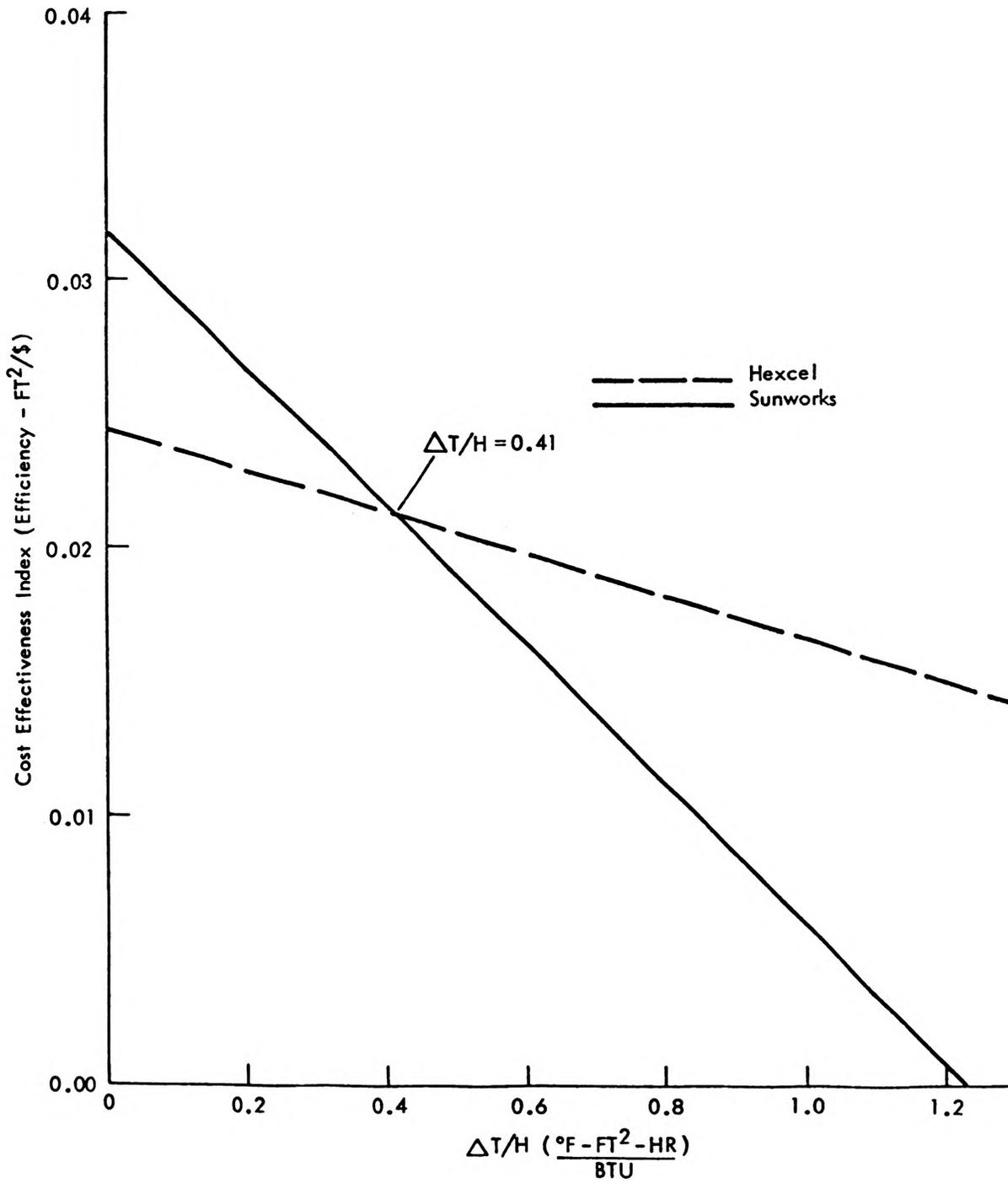
Figure 1 - Cost Effectiveness Index Versus  $\Delta T/H$  Plots for Sunworks and Hexcel Collectors
