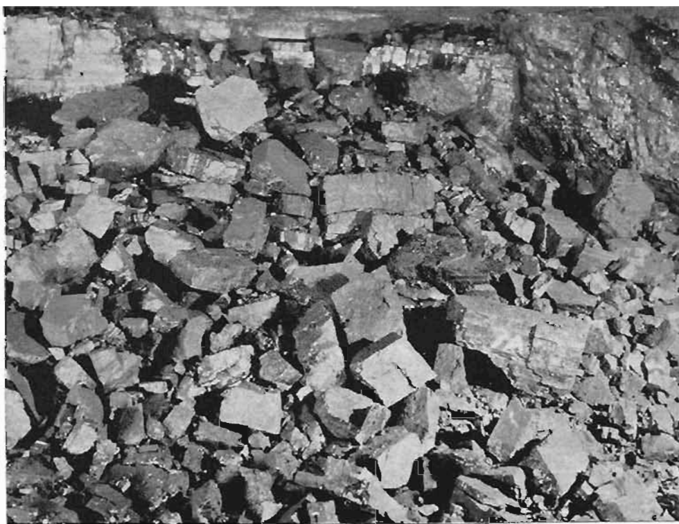
View showing coal dislodged by Cardox bleasting method.
