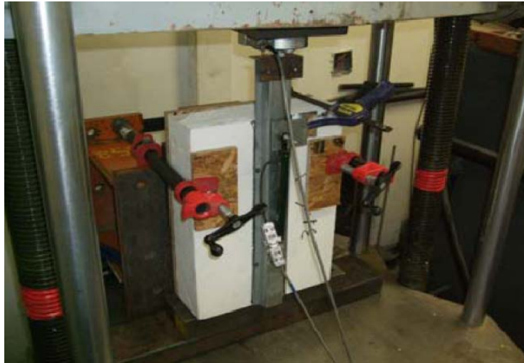
Figure 3.2. Typical shear test set-up (PEI, 2010a).
