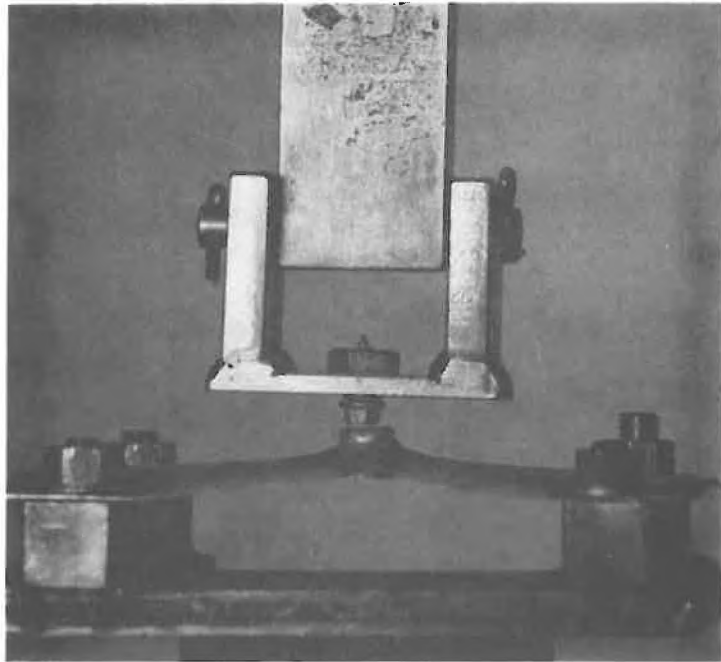
A-VII(c) Conventional Failure Mode in .060 in. Thick Sheet. Note the Slight Overall Sheet Deformation, Localize Necking and Tensile Sheet Failure.
