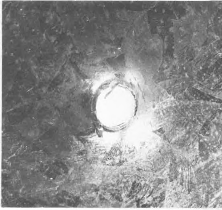
A-VII(k) At Failure the Sheet Experienced Extremely Local Bending and Partial Shearing of Some Material Around the Periphery of the Hole.
