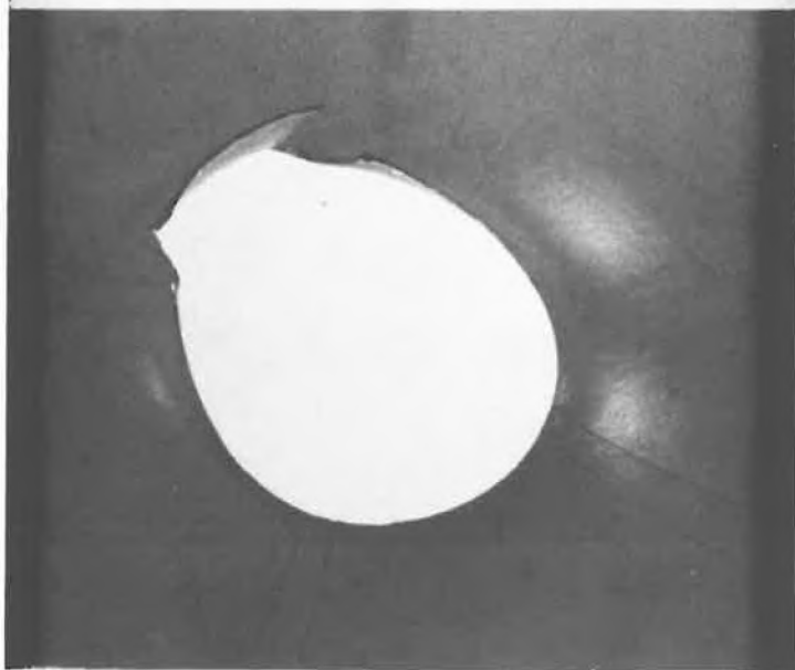
A-VII(f) Punch-Out Failure in .022 in. Thick Sheet.
