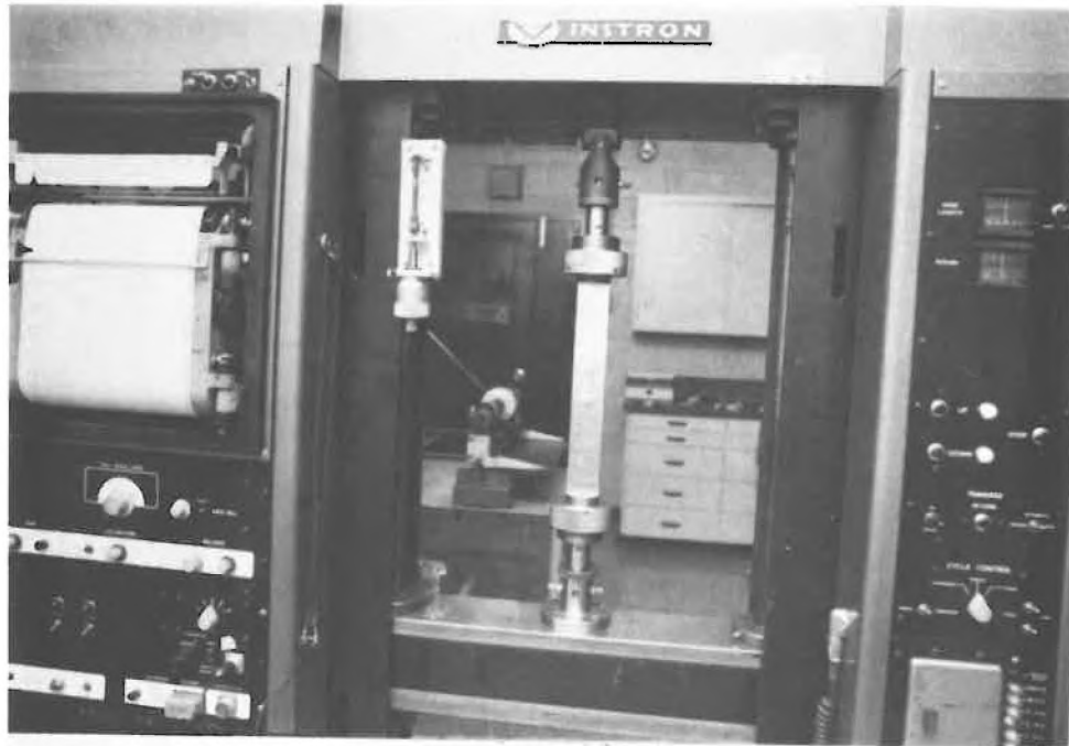
A-VII (m) Static Shear Test Sample, Installed in Tensile Testing Machine.
