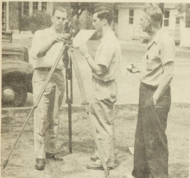
Taking a solar observation with a wild theodolite over Station C erected by Veterans of World War I, just south of the gym is E. A. Weinel, '44, Jim Fisher, '48, and Professor Carlton.
