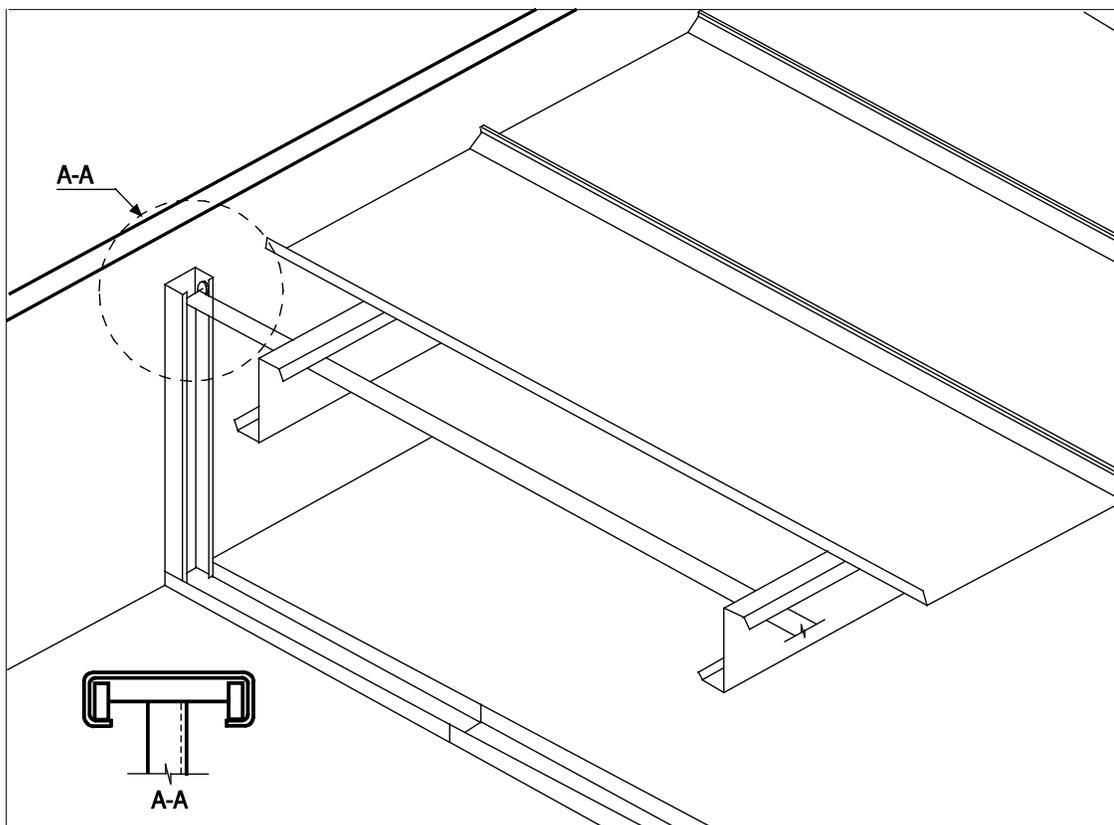
**Figure 2 - Example of Lateral Restraint Test Device**
