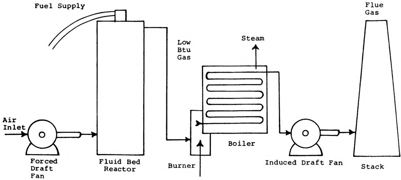
Figure II. Schematic of a Gasification Unit.
