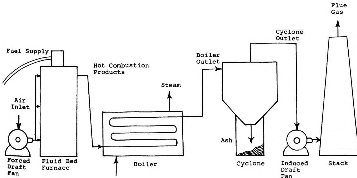
Figure I. Schematic of a Fluidized-Bed Combustion Module.
