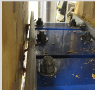
Figure C-1 Photograph of Clamping System
