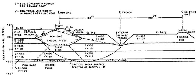
FIGURE 4-SOIL PROFILE AND DIKE STABILITY-STAGE 1
