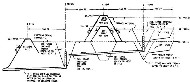
FIGURE 2-DIKE AND TRENCH CROSS-SECTION
