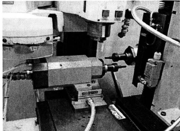
Figure 3: High speed spindles and mill tooling.
