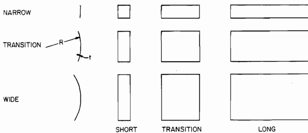
Fig. 2.2 Ranges of Possible Curved Plate Geometries<sup>21</sup>
