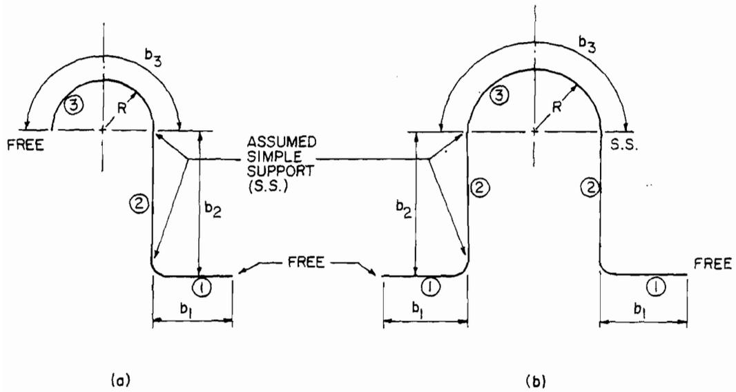
Fig. 2.6 Typical Cross-Sections Consisting of Flat and Curved Elements.
