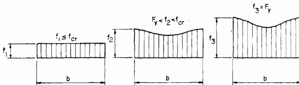
Fig. 2.7 Consecutive Stages of Stress Distribution in Stiffened Compression Elements.<sup>30</sup>
