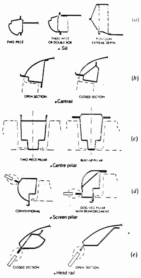
Fig. 1.1 Typical Car Body Member Sections<sup>3</sup>
