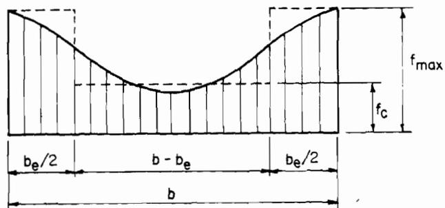
Fig. 2.9 Effective Width of a Curved Compression Element<sup>38</sup>
