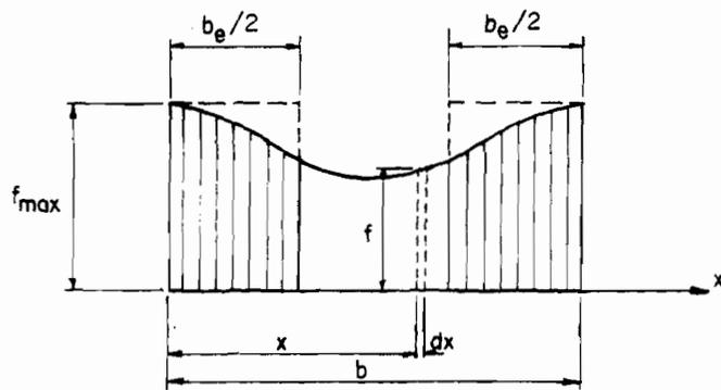
Fig. 2.8 Effective Width of a Stiffened
