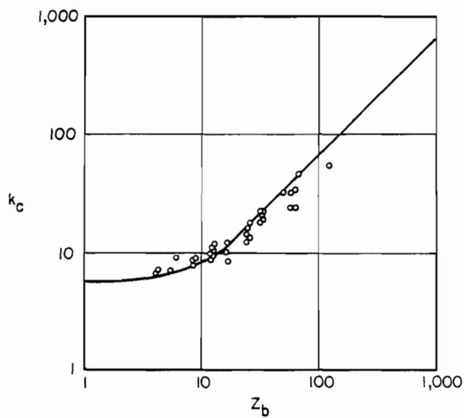
Fig. 2.1 Comparison of Test Data With Theory for Axially Compressed Curved Plates.<sup>21</sup>
