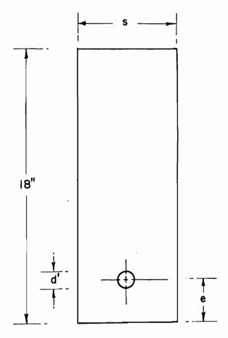
Figure 1. Definition of Symbols used in Table 3a
