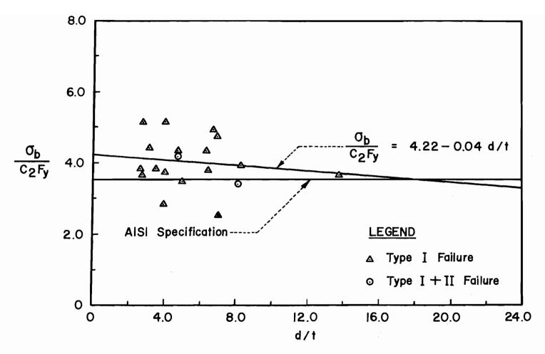
Fig. 15 Effect of d/t on Lonitudinal Shear Strength of Steel Sheets (Double Shear e/d = 2.5)<sup>6,9,10</sup>
