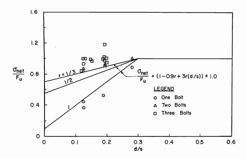
Fig. 5 (c) Effect of d/s on Tensile Strength of Bolted Connections (Single Shear,  $Multi-Bolt)^{13}$
