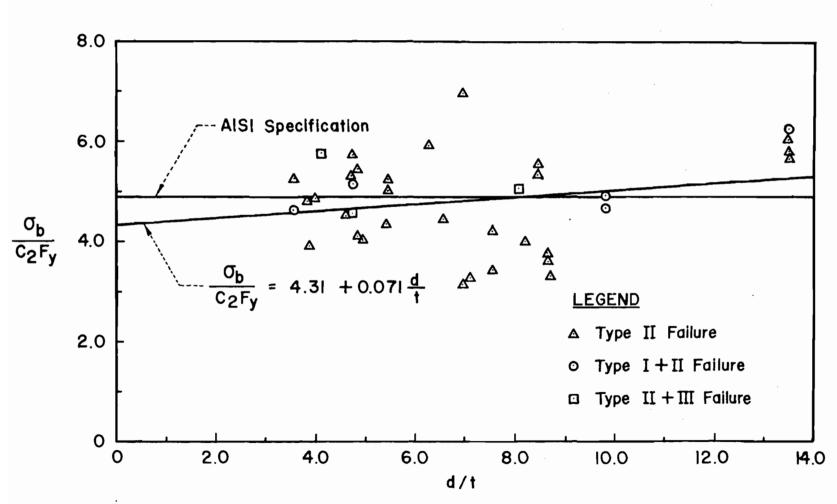
Fig. 6 Effect of d/t Ratio on Bearing Strength (Single Shear)  $^{6,7,9,10,14}$
