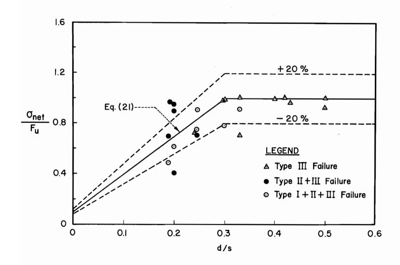
Fig. 18 Effect of d/s on Tensile Strength of Bolted Connections Using Low Ductility Steels (Single Shear, One Bolt)<sup>6</sup>
