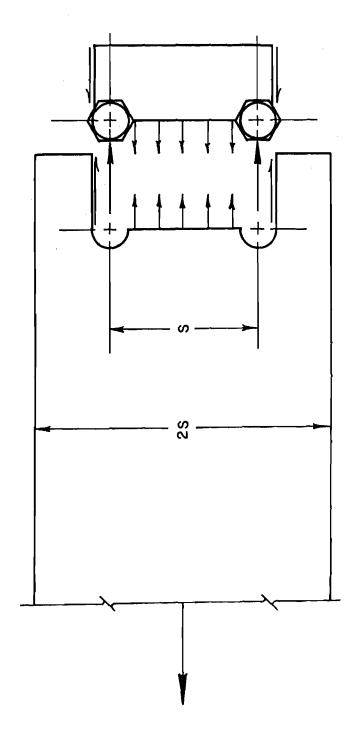
Figure 28. Failure Mode Governed by Combined Shear and Tension
