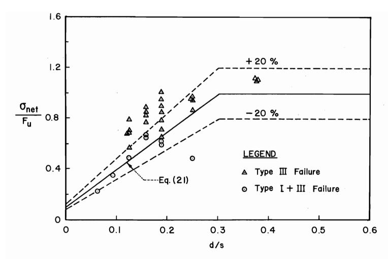
Fig. 20 Effect of d/s on Tensile Strength of Bolted Connections Using High Ductility Steels (Double Shear, One Bolt) 9,10
