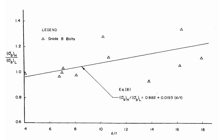
Figure 12. Effect of d/t on the Ratio of  $(\sigma_b)_H/(\sigma_b)_L$  for Single Shear Connections without Washers, Grade 8 Bolts
