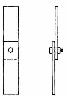
Figure 2. Test Assembly for Single Shear Connections
