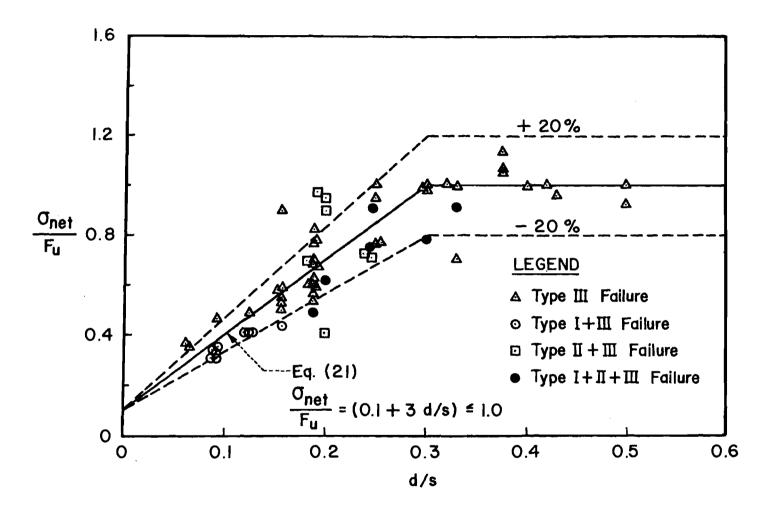
Fig. 19 Effect of d/s on Tensile Strength of Bolted Connections (Combination of the Data Shown in Figs. 17 and 18) (Single Shear, One Bolt)<sup>6,9,10</sup>
