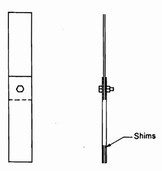
Fig. 22 Double Shear Connection
