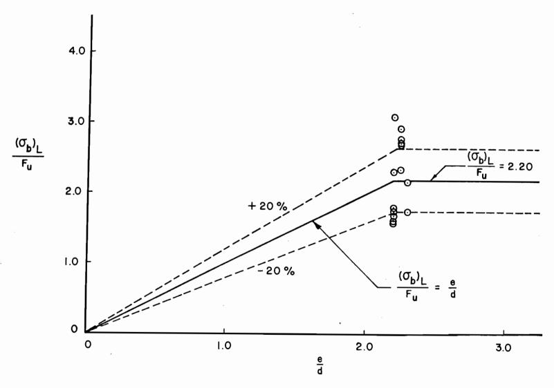
Figure 17. Correlation Between the Predicted Ultimate Bearing Stress and Test Data Single Shear Connections without Washers,  $\frac{F_u}{F_y} \ge 1.15$ ,  $0.036 \le t < \frac{3}{16}$  in.
