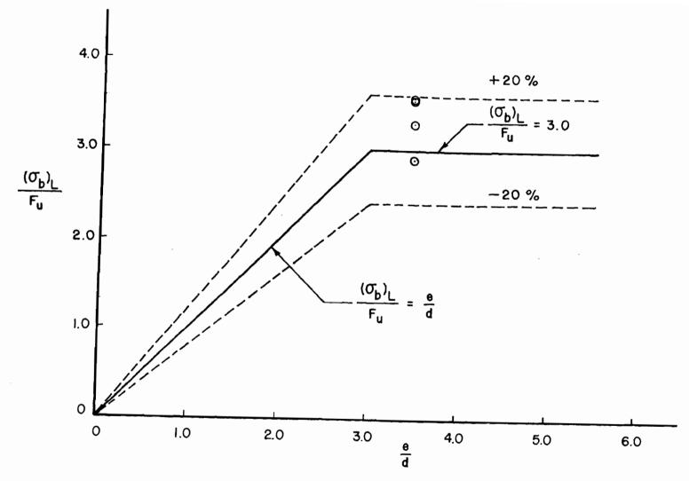
Figure 23. Correlation Between the Predicted Ultimate Bearing Stress and Test Data Double Shear Connections with Washers,  $\frac{F_u}{F_y} \le 1.15$ , t < 0.024 in.
