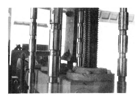
Figure 5. Photographs of the Typical Failure Modes due to Excessive Bolt Rotation and Dishing of Steel Sheets
