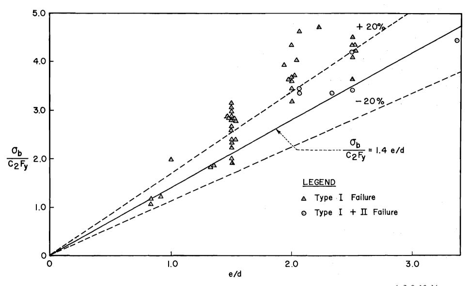
Fig. 10 Effect of e/d on Longitudinal Shear Strength of Steel Sheets (Single Shear)<sup>6,7,9,10,14</sup>
