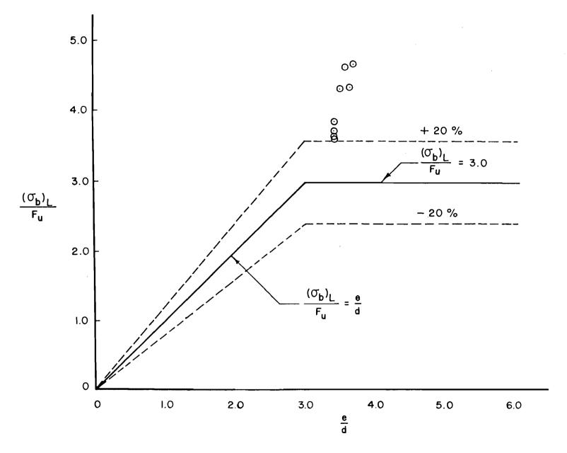
Figure 20. Correlation Between the Predicted Ultimate Bearing Stress and Test Data Double Shear Connections without Washers,  $\frac{F_u}{F_y} < 1.15$ , 0.036  $\leq t < \frac{3}{16}$  in.
