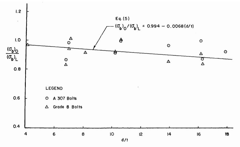
Figure 9. Effect of d/t on the Ratio of  $(\sigma_b)_0/(\sigma_b)_L$  for Double Shear Connections without Washers
