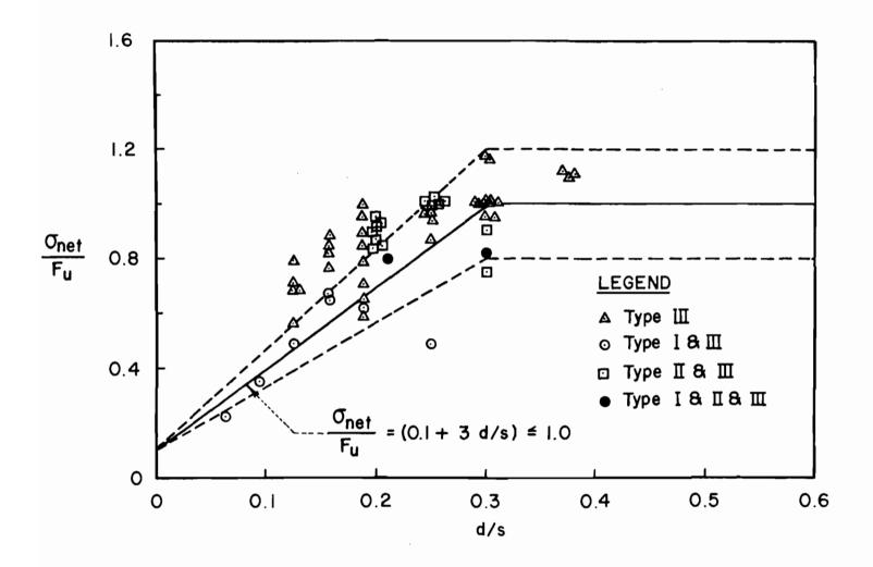
Fig. 5 (a) Effect of d/s on Tensile Strength  $\alpha f$  Bolted Connections with Washers (Double Shear, One Bolt)
