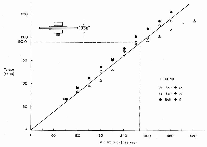
Fig. 19 Relationship of Torque vs. Nut Rotation for 5/8 in. \$\phiA325\$ Bolts
