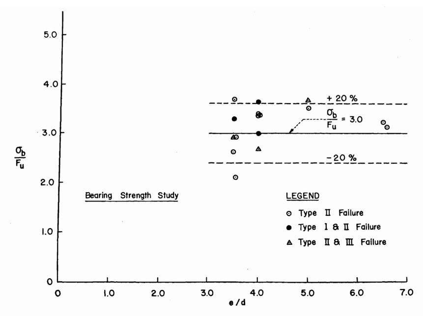
Fig. 10 Single Shear Connections with Washers,  $F_u/F_y \le 1.15$ ,  $e/d \ge 3.5$
