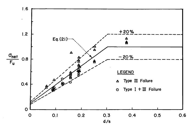
Fig. 17 Effect of d/s on Tensile Strength of Bolted Connections
