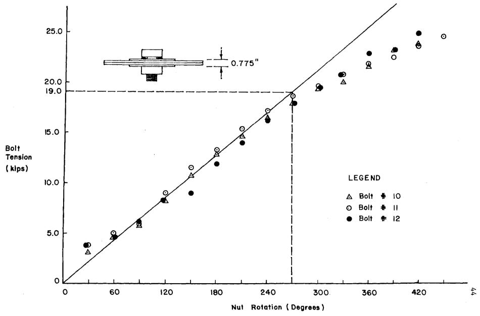
Fig. 10 Relationship of Bolt Tension vs. Nut Rotation for 5/8 in. \$\phi A325 Bolts
