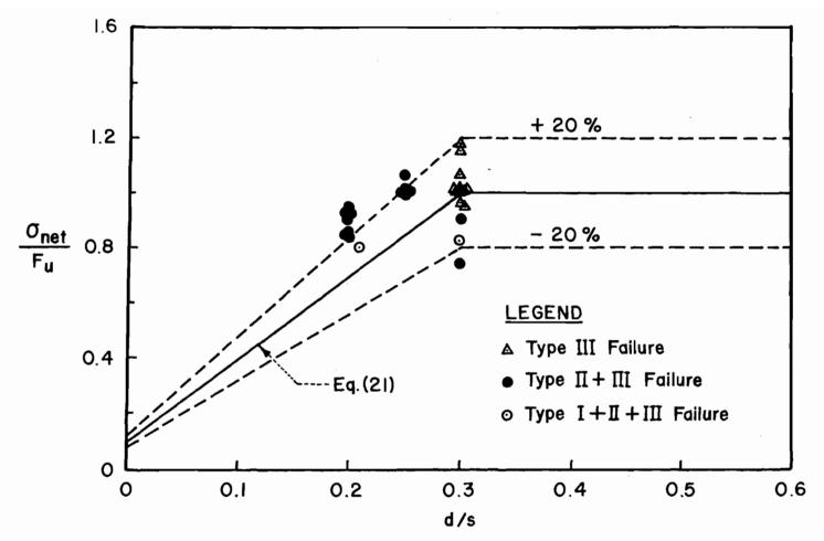
Fig. 21 Effects of d/s on Tensile Strength of Bolted Connections Using Low Ductility Steels (Double Shear, One Bolt) $^6$
