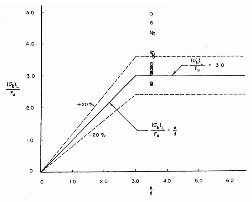
Figure 19. Correlation Between the Predicted Ultimate Bearing Stress and Test Data Double Shear Connections without Washers,  $\frac{F_u}{F_y} \ge 1.15$ ,  $0.036 \le t < \frac{3}{16}$  in.
