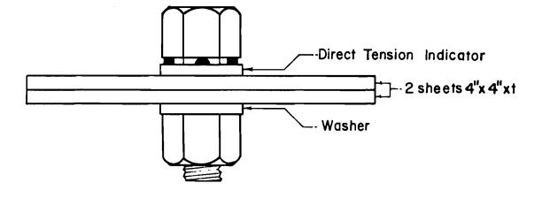
Fig. 5 Pretension Test Assembly
