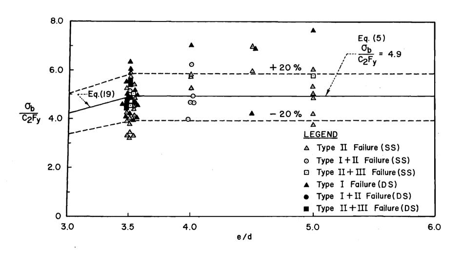
Fig. 5 Effect of Single and Double Shear Connections on Bearing Strength 9,10
