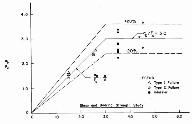
Fig. 24 Single Shear Connections with Washers,  $F_u/F_y \ge 1.15$ ,  $t \le 0.036$  in.
