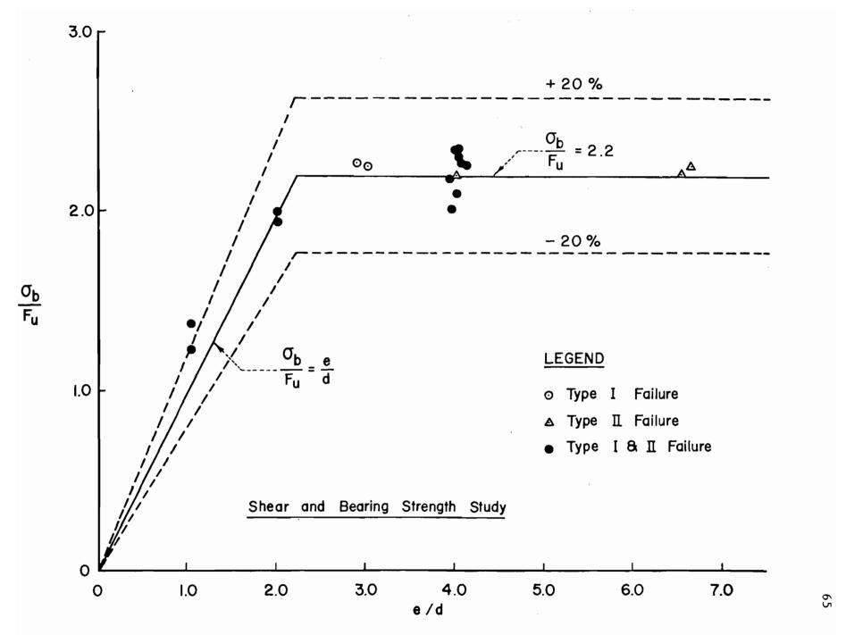
Fig. 11 Single Shear Connections without Washers,  $F_u/F_y \ge 1.15$
