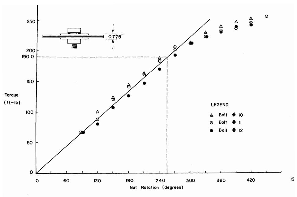
Fig. 18 Relationship of Torque vs. Nut Rotation for 5/8 in. \$\phiA325\$ Bolts
