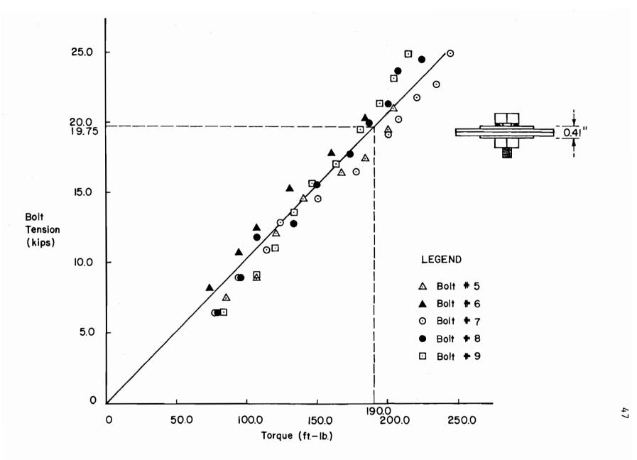
Fig. 13 Relationship of Bolt Tension vs. Torque for 5/8 in. \$\phiA325\$ Bolts
