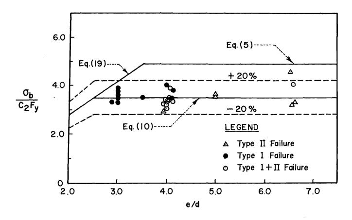
Fig. 9 Effect of e/d on Bearing Strength of Bolted Connections without Washers  $^{7}$
