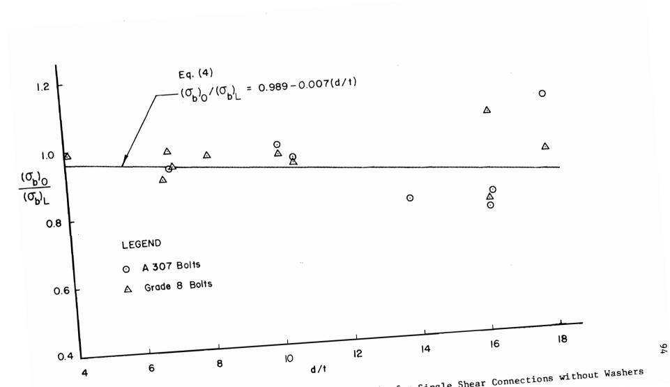
Figure 8. Effect of d/t on the Ratio of  $(\sigma_b)_0/(\sigma_b)_L$  for Single Shear Connections without Washers
