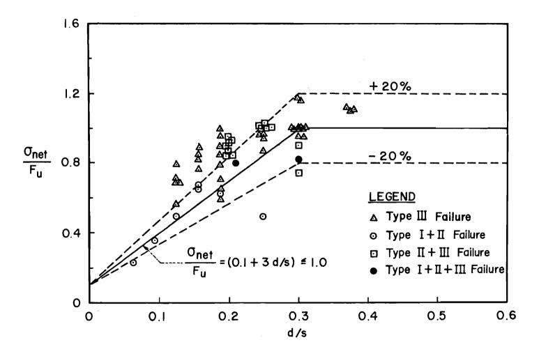
Fig. 22 Effect of d/s on Tensile Strength of Bolted Connections (Combination of the Data Shown in Figs. 20 and 21) (Double Shear, One Bolt) $^{6,9,10}$
