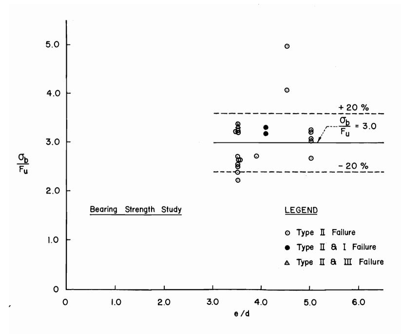
Fig. 9 Single Shear Connections with Washers,  $F_u/F_y \ge 1.15$ ,  $e/d \ge 3.5$
