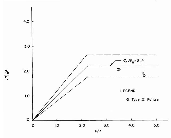
Fig. 28 Double Shear Connections Without Washers  $F_u/F_y \ge 1.15$ ,  $t \le 0.036$  in.
