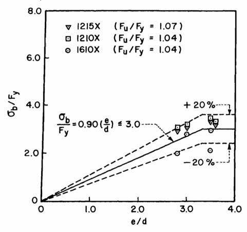
Fig. 3 Effect of Ductility  $(F_u/F_y \le 1.1)^6$
