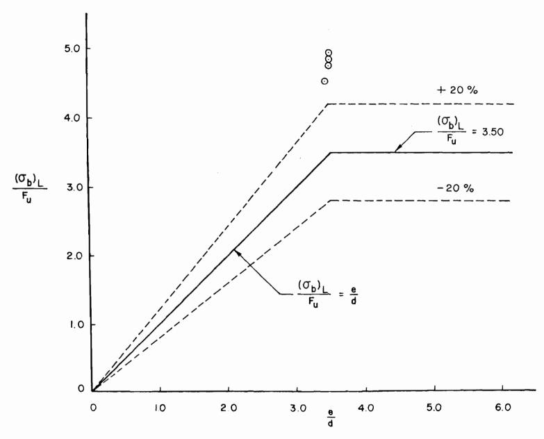
Figure 22. Correlation Between the Predicted Ultimate Bearing Stress and Test Data Double Shear Connections with Washers,  $\frac{F_u}{F_y} \ge 1.15$ , t  $\le 0.024$  in.
