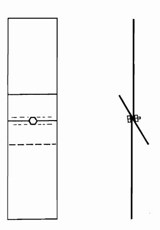
Fig. 26 Failure by Bolt Rotation and Sheet Warping
