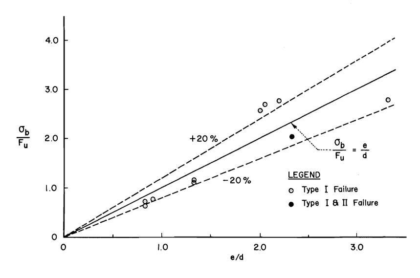
Fig. 3 Single Shear Connections with Washers, F  $_{\!\!u}/{\rm F}_{\!\!y}$   $^<$  1.15, e/d  $^<$  3.5, Shear Strength Study
