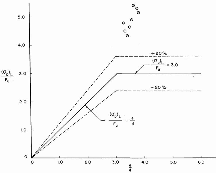
Figure 16. Correlation Between the Predicted Ultimate Bearing Stress and Test Data Double Shear Connections with Washers,  $\frac{F_u}{F_y}$  <1.15, 0.024  $\leq$  t  $< \frac{3}{16}$  in.
