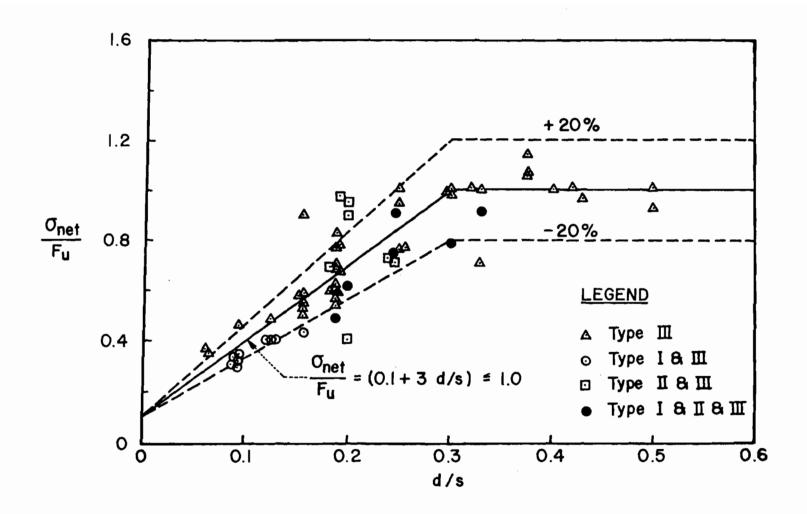
Fig. 5 (b) Effect of d/s on Tensile Strength of Bolted Connections with Washers (Single Shear, One Bolt)
