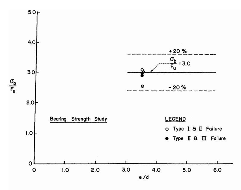
Fig. 8 Double Shear Connections with Washers,  $F_u/F_y < 1.15$ ,  $e/d \ge 3.5$
