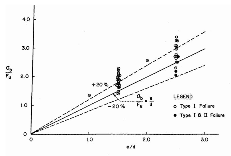
Fig. 2. Double Shear Connections with Washers,  $\frac{F_u}{F_y} \ge 1.15$ , e/d < 3.5, Shear Strength Study
