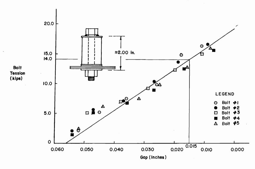
Fig. 6 Calibration of Direct Tension Indicator
