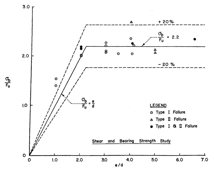
Fig. 12 Single Shear Connections without Washers,  $F_u/F_y < 1.15$ ,  $t \ge 0.036$  in.
