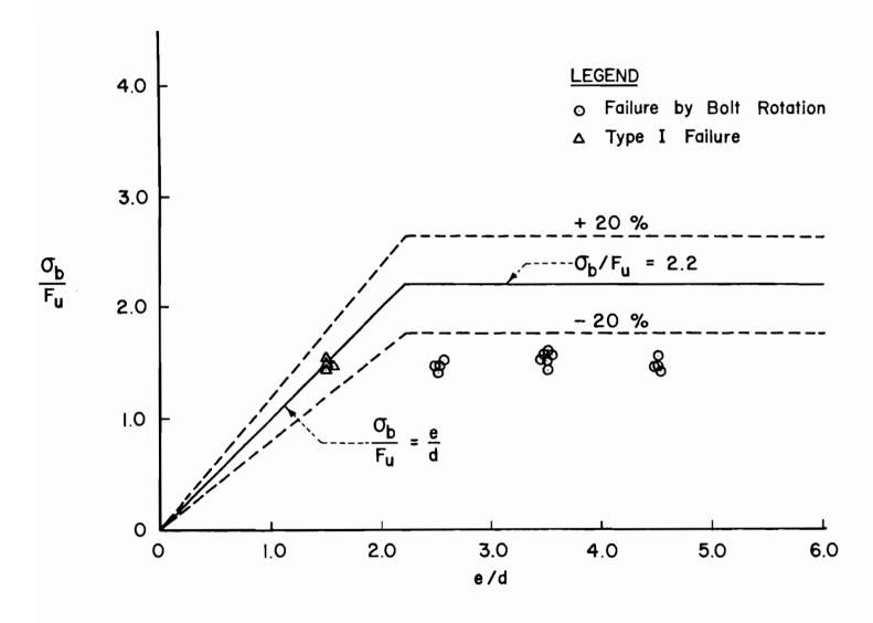
Fig. 15 Single Shear Connections without Washers,  $F_u/F_y \ge 1.15$ ,  $t \le 0.036$  in.
