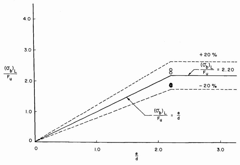
Figure 18. Correlation Between the Predicted Ultimate Bearing Stress and Test Data Single Shear Connections Without Washers,  $\frac{F_u}{F_y} < 1.15$ ,  $0.036 \le t < \frac{3}{16}$  in.
