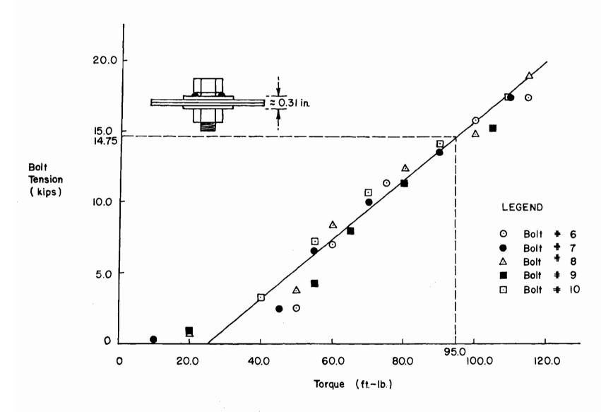
Fig. 12 Relationship of Bolt Tension vs. Torque for 1/2 in.  $\phi A325$  Bolts
