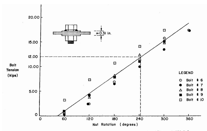
Fig. 8 Relationship of Bolt Tension vs. Nut Rotation for 1/2 in.  $\phi A325$  Bolts
