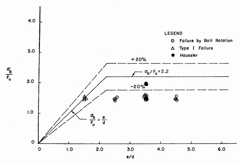
Fig. 25 Single Shear Connections without Washers,  $F_u/F_y \ge 1.15$ ,  $t \le 0.036$  in.
