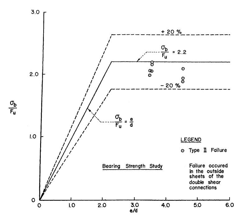
Fig. 14 Double Shear Connections without Washers,  $F_u/F_y \ge 1.15$ ,  $t \ge 0.036$  in.
