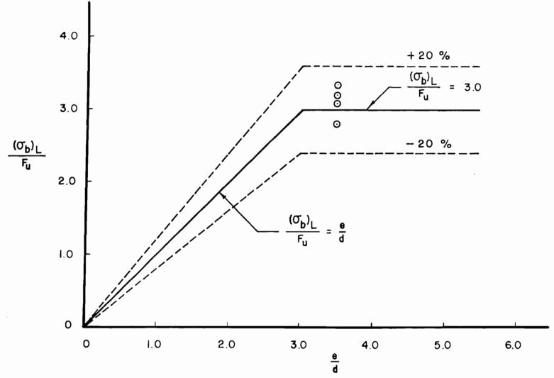
Figure 27. Correlation Between the Predicted Ultimate Bearing Stress and Test Data Double Shear Connections without Washers,  $\frac{F_u}{F_y} < 1.15$ , t < 0.036 in.
