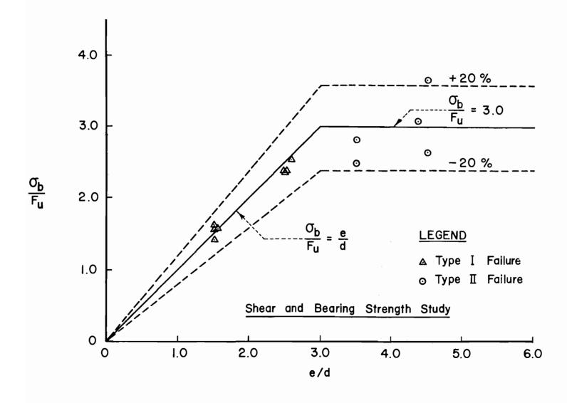
Fig. 13 Single Shear Connections with Washers,  $F_u/F_y \ge 1.15$ ,  $t \le 0.036$  in.
