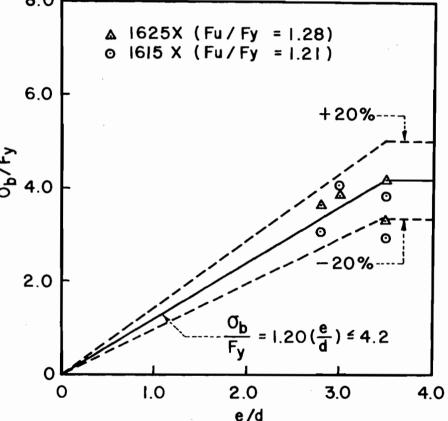
Fig. 2 Effect of Ductility  $(F_u/F_y \sim 1.25)^6$
