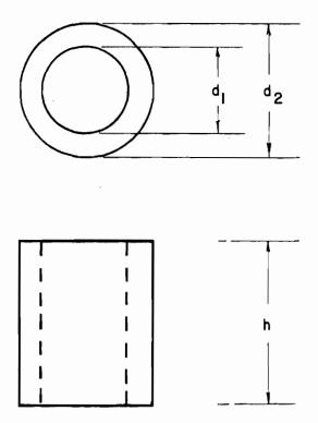
Fig. 1 Load Cell Dimensions
