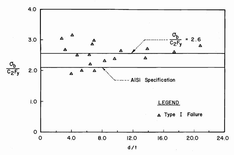
Fig. 12 Effect of d/t on Longitudinal Shear Strength of Steel Sheets (Single Shear, e/d = 1.5)<sup>9,10</sup>
