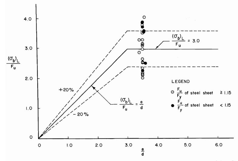
Figure 14. Correlation Between the Predicted Ultimate Bearing Stress and Test Data Single Shear Connections with Washers,  $0.024 \le t < \frac{3}{16}$  in.
