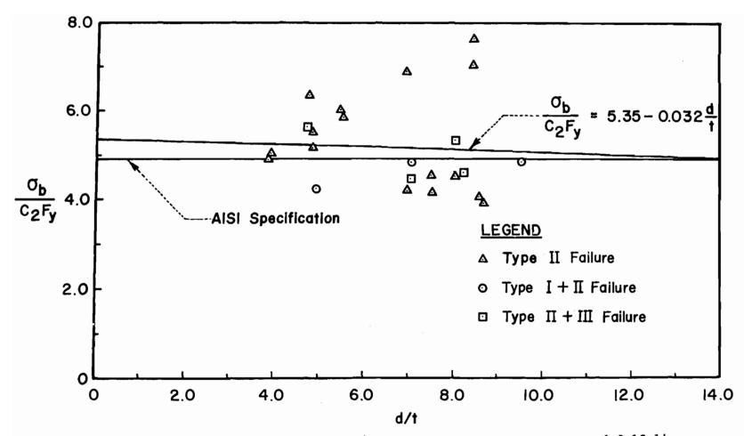
Fig. 7 Effect of d/t Ratio on Bearing Strength (Double Shear)<sup>6,9,10,14</sup>
