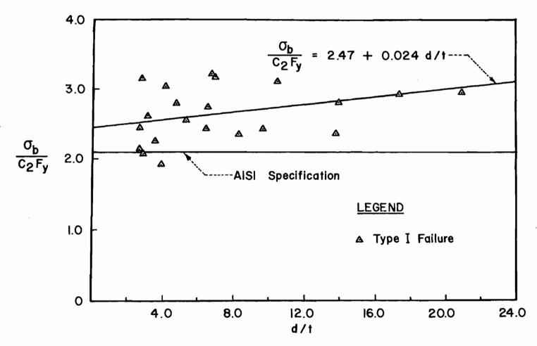
Fig. 13 Effect of d/t on Longitudinal Shear Strength of Steel Sheets (Double Shear, e/d = 1.5)<sup>9,10</sup>
