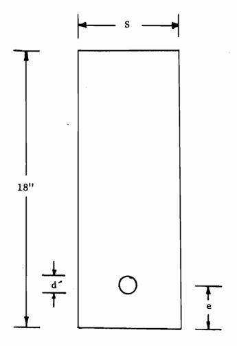
Fig. 20 Test Specimen Blanks
