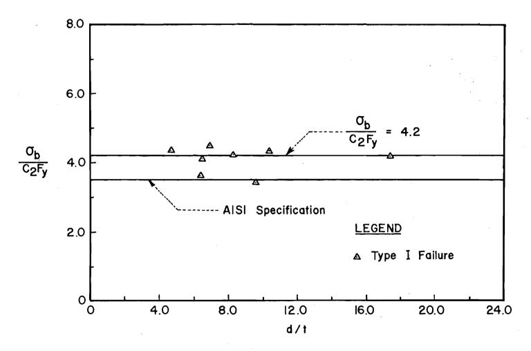
Fig. 14 Effect of d/t on Longitudinal Shear Strength of Steel Sheets (Single Shear, e/d = 2.5)<sup>9,10</sup>
