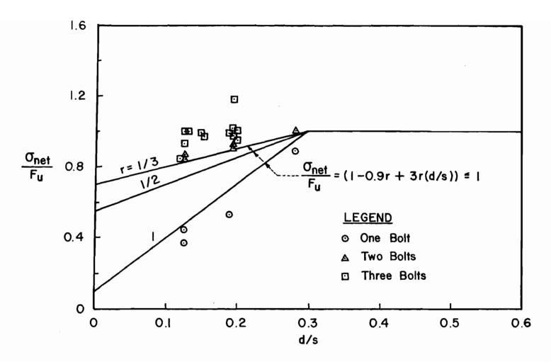
Fig. 23 Effect of d/s on Tensile Strength of Bolted Connections (Single Shear, Multi-Bolt)<sup>5</sup>
