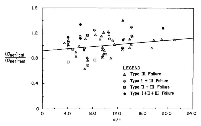
Fig. 24 Effect of d/t on Tensile Strength of Bolted Connections (Single Shear) $^{6,9,10}$
