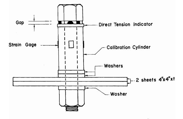
Fig. 4 Pretension Test Assembly Used for Calibrating Direct Tension Indicator
