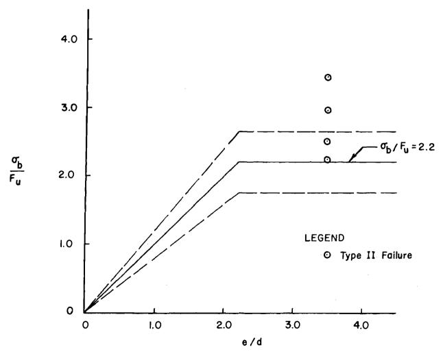
Fig. 27 Single Shear Connections Without Washers  $\frac{F_u}{F_y} \ge 1.15$ ,  $t \ge 0.036$  in.
