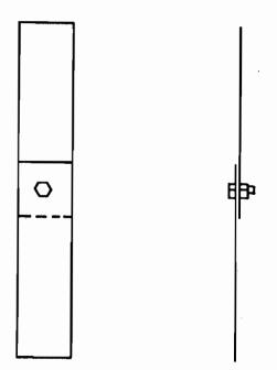
Fig. 21 Single Shear Connection
