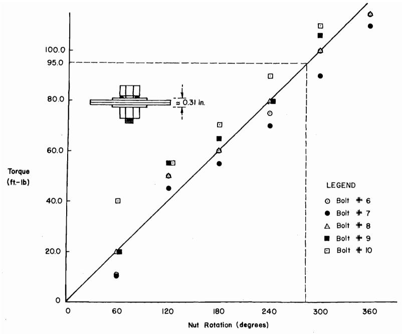
Fig. 16 Relationship of Torque vs. Nut Rotation for 1/2 in. φA325 Bolts
