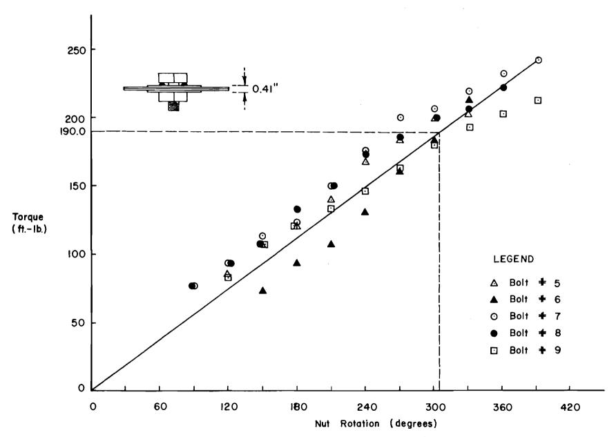
Fig. 17 Relationship of Torque vs. Nut Rotation for 5/8 in.  $\phi A325$  Bolts
