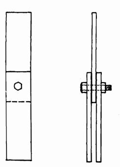
Figure 3. Test Assembly for Double Shear Connections
