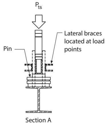
**Figure 2 - Section of Simply Supported Beam Test**
