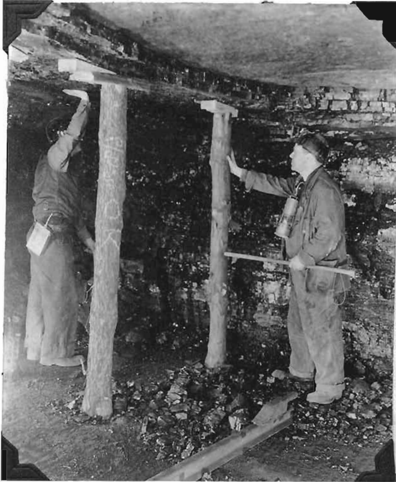
CAREFUL EXAMINATION OF ROOF NECESSARY Note mine foreman carries flame safety lamp, sounding rod, and wears electric cap lamp. Note also block used for blocking mine cars at the face.
