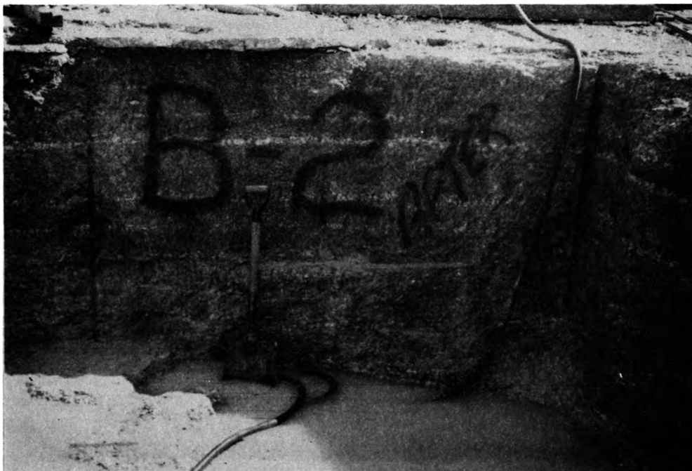
Figure E-14. Bench for Test B-2 After Blasting
