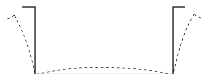
Figure C-C3.1.2.1-4 Lateral Buckling of U-Shaped Beam
