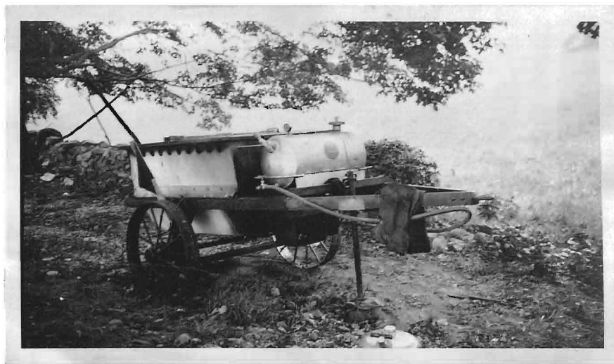
Kerosene Fired Melting Kettle for Heating Enamel
