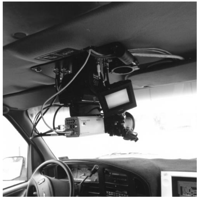
FIGURE 3 Cab-mounted video camera in data collection vehicle.
