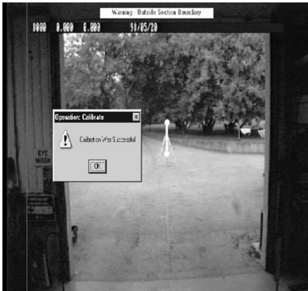
FIGURE 8 Image used to calibrate Surveyor camera.
