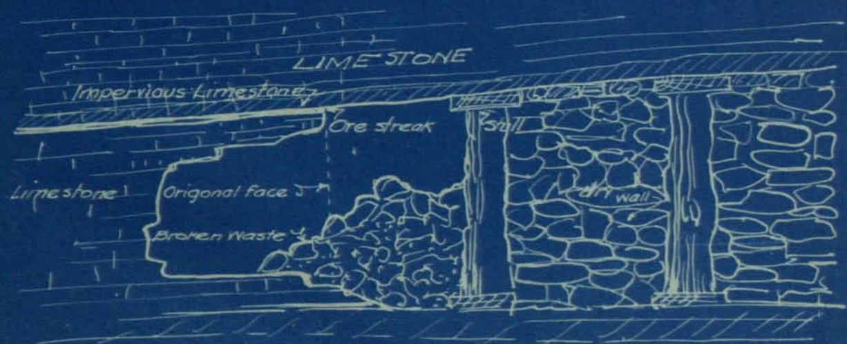
SECTION THRU STOPE SHOWING ORE STREAK AND GIVING METHODS OF EXTRACTION.
