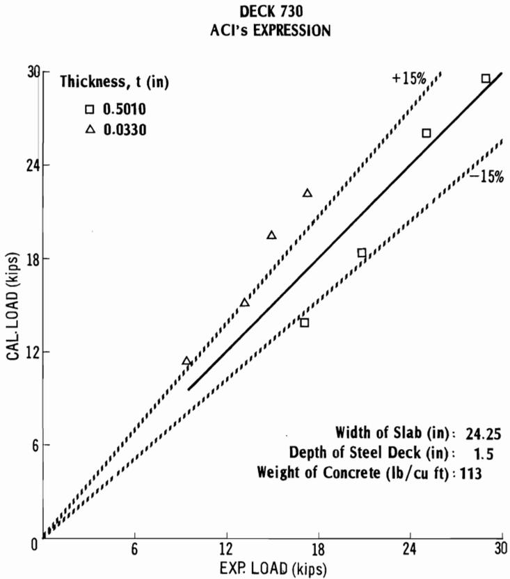
Fig. 5b - EXPerimental and CALculated Ultimate Shear-Bond Capacities of Deck-730, Eq. (2), Step II.
