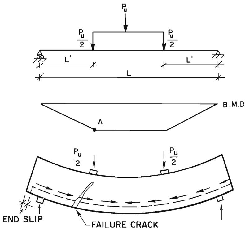
Fig. 2 - Typical Shear-Bond Failure
