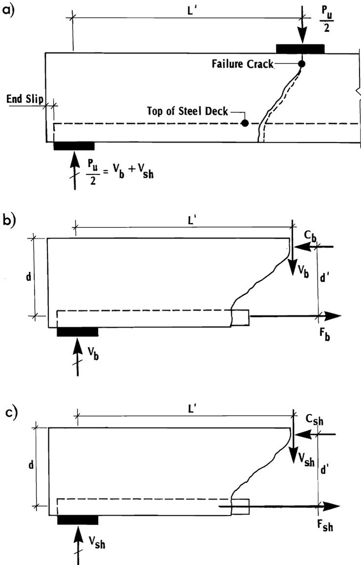
Fig. 3 - Internal Forces at Region of Crack
