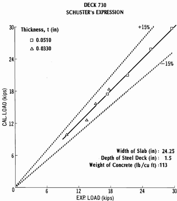
Fig. 4a - EXPerimental and CALculated Ultimate Shear-Bond Capacities of Deck-730, Eq. (1), Step I.
