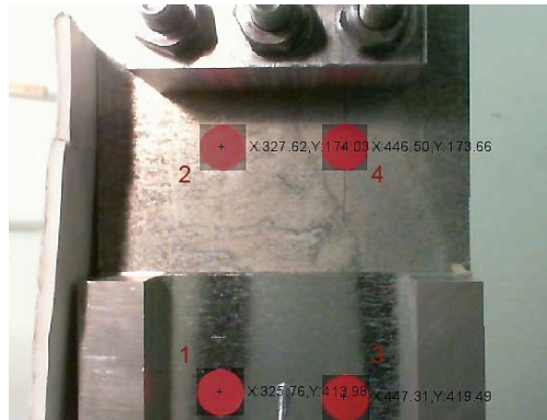
Figure 5: Matlab frame-by-frame post-processing of the displacement video camera
