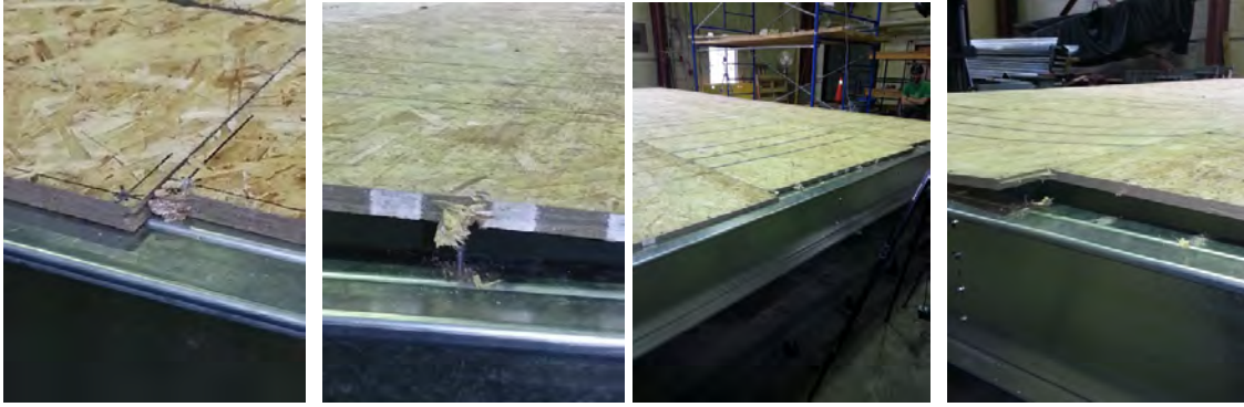
(a) Deformation from monotonic loading
