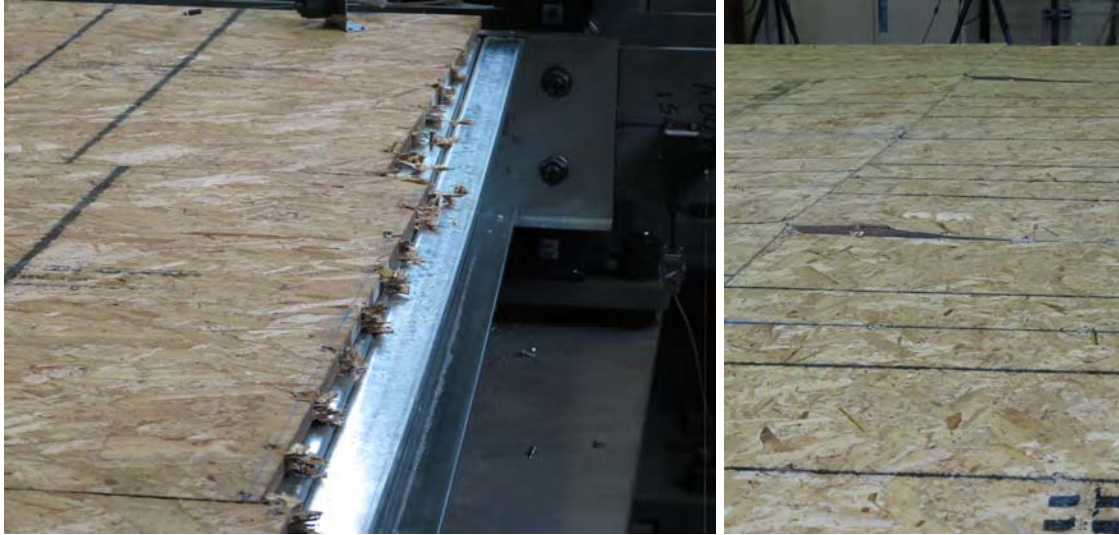
(b) Diaphragm behaviour from cyclic loading
