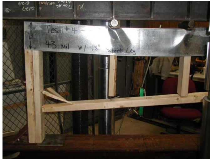
Figure 8 – 43 mil L-Header Assembly at Failure Load
