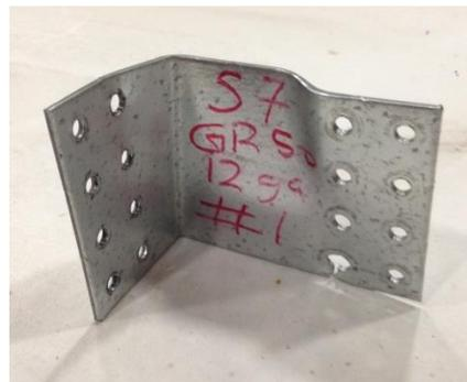
Figure 2.6: Test result of clip angle S7 #1
