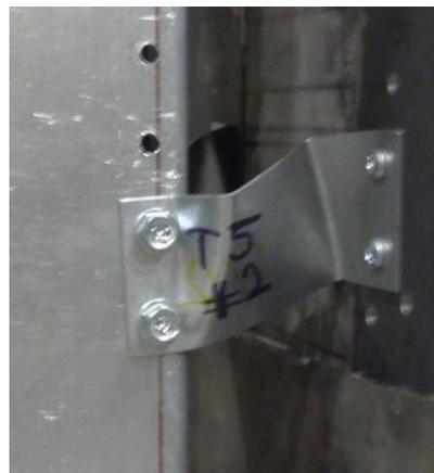
Figure 2.4: Test result of clip angle T5a #2
