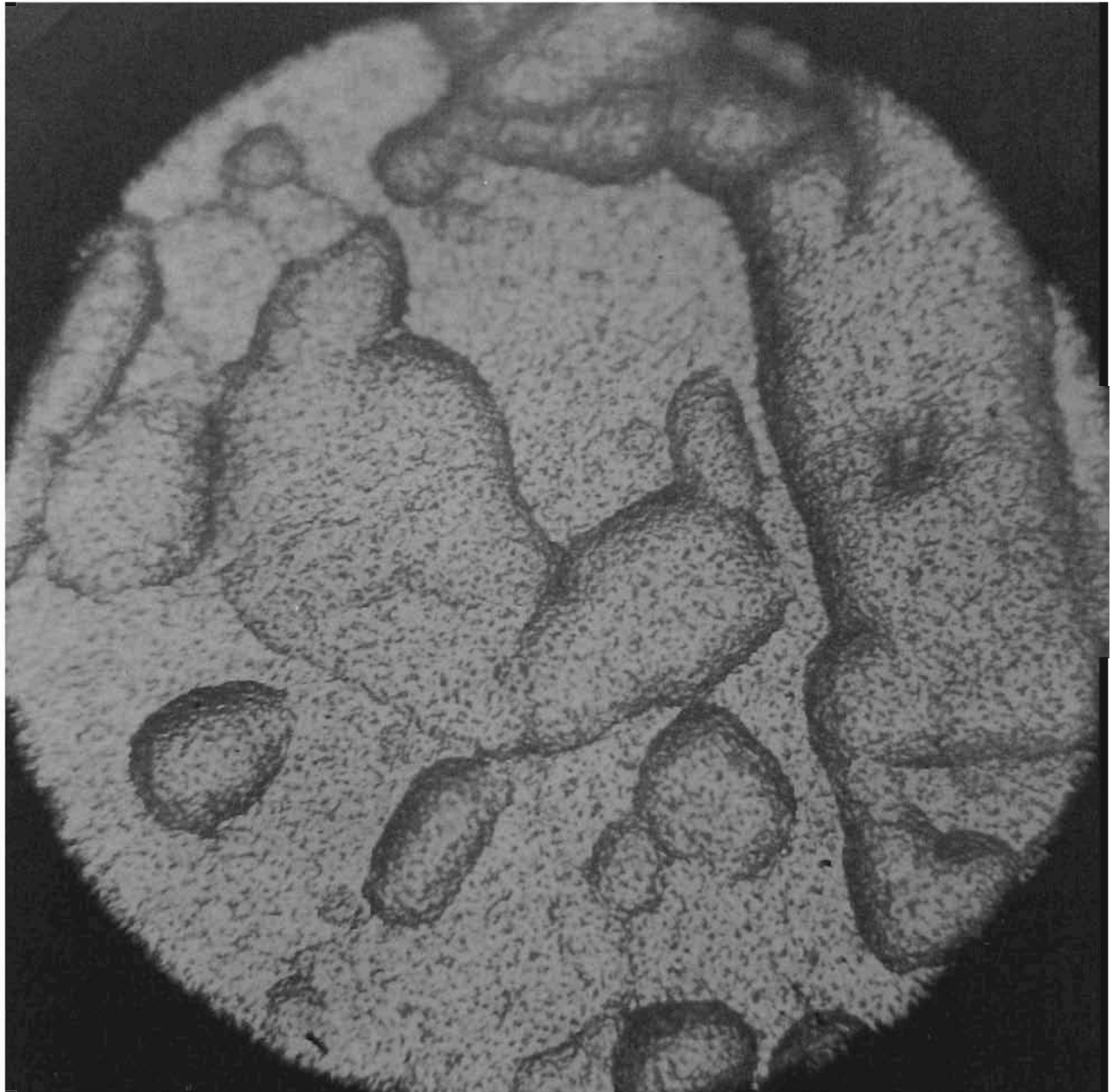
Figure 15.- Nickel deposit at 150X; pH of catholyte, 5.40.
