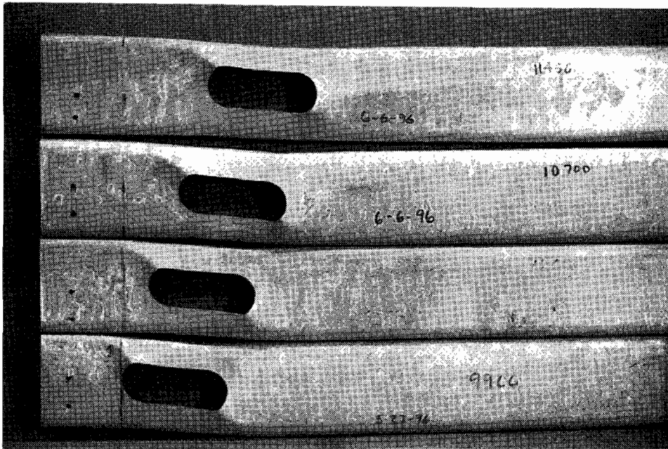
Figure 12 Failed Beam Test Specimens (3.625" with Elliptical Hole)
