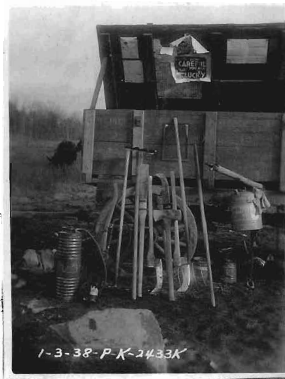
Tools used in the final marginal conditioning operations. From left to right: "air-oil" wood burner, mower tooth or fire rake, horse made topping blade, double blade bush hooks, ax, and pitch fork for piling growth for burning.
