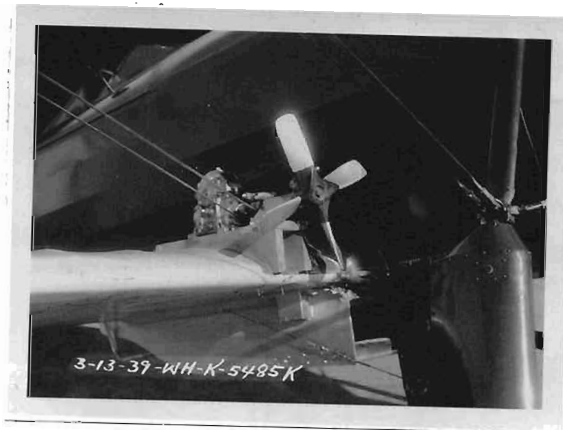
Close up view showing agitator drive, venturi and arm to dust release valve.
