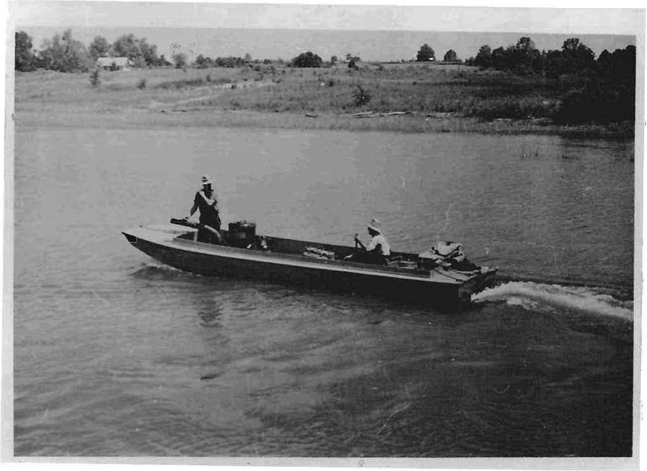
Larvicidal boat equipped with power dust blower
