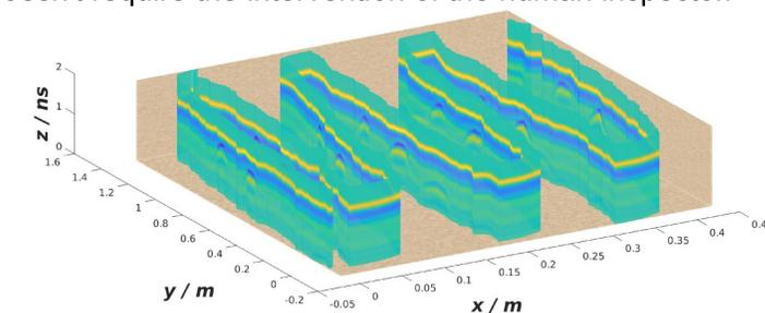
Fig. 3. The B-scan profile tagged with metric positioning information.
