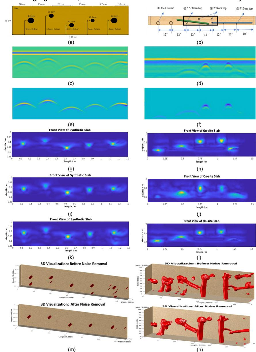
Fig. 2. Effectiveness and noise comparison of proposed method on both synthetic and field GPR data
