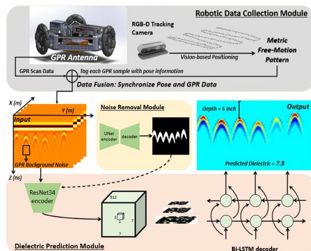
Fig. 1. The system architecture consists of a robotic GPR data collection module and a DNN-based GPR data analysis module.
