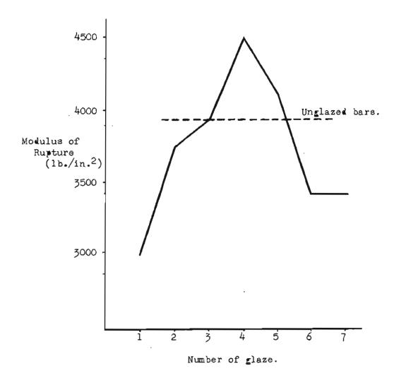
CHANGE IN MODULUS OF RUPTURE WITH CHANGE IN GLAZE COMPOSITION.
