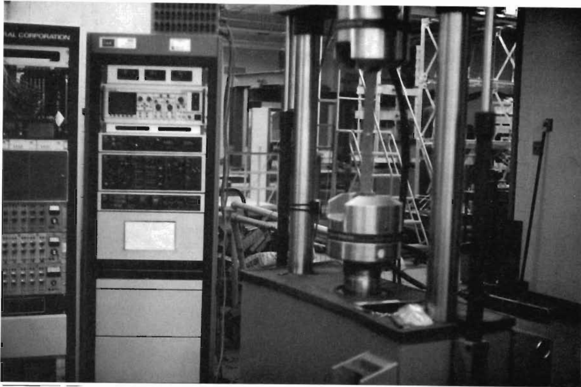
Figure 3.1 Photo of Materials Test System 880 Tension Testing Machine
