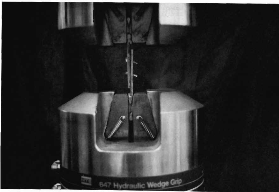
Figure 3.6 Screw Tilting and Plate Separation During Shear Test
