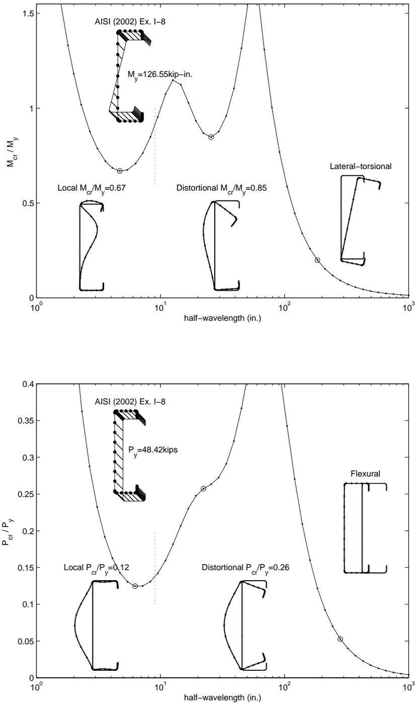
(a) 9CS2.5x059 of AISI 2002 Cold-Formed Steel Design Manual Example I-8
