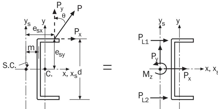
Figure C-D3.2.2-6 C-Section Member Subjected to a Concentrated Load
