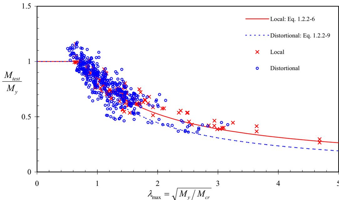
**Figure C-1.2.2-2 Direct Strength Method for laterally braced beams**
