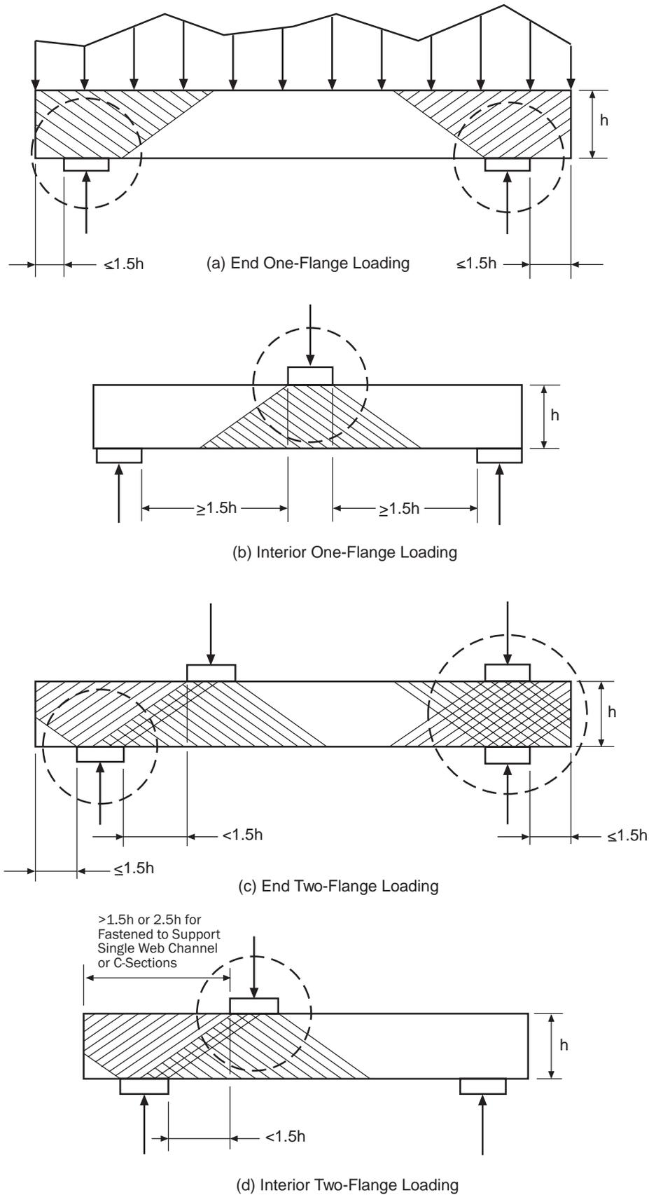
Figure C-C3.4.1-4 Assumed Distribution of Reaction or Load
