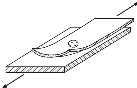
Figure C-E2.2.1.2-1 Out of Plane Distortion of Welded Connection
