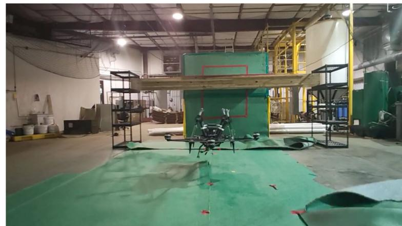
Clamping tests show that arms on top of BIRDS can clamp on a girder above and the clamping mechanism can hold the total weight of BIRDS:
