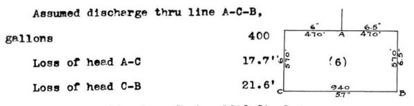
Equivalent diameter of pipe,1980 ft. long, which will give a loss of head of 39.3 feet when discharging 400 gallons,is 5.8 inches. Assumed loss of head from A to B,20' Discharge thru line A-B,gallons 520 Discharge thru line A-C-B,gal's 270
