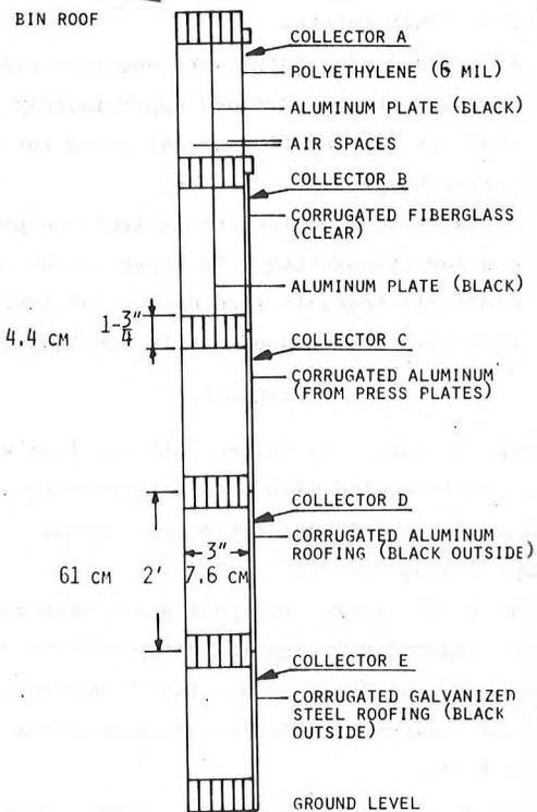
Figure 1. Collector Detail, Redfield Solar Bin.
