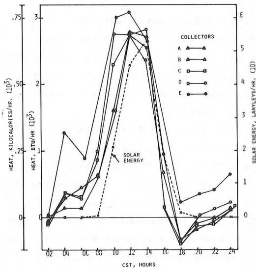
Figure 2. Average Hourly Heat Collection and Solar Energy on a Horizontal Surface. Note: Values for Collector E are distorted due to heat transfer from plenum through bin wall.
