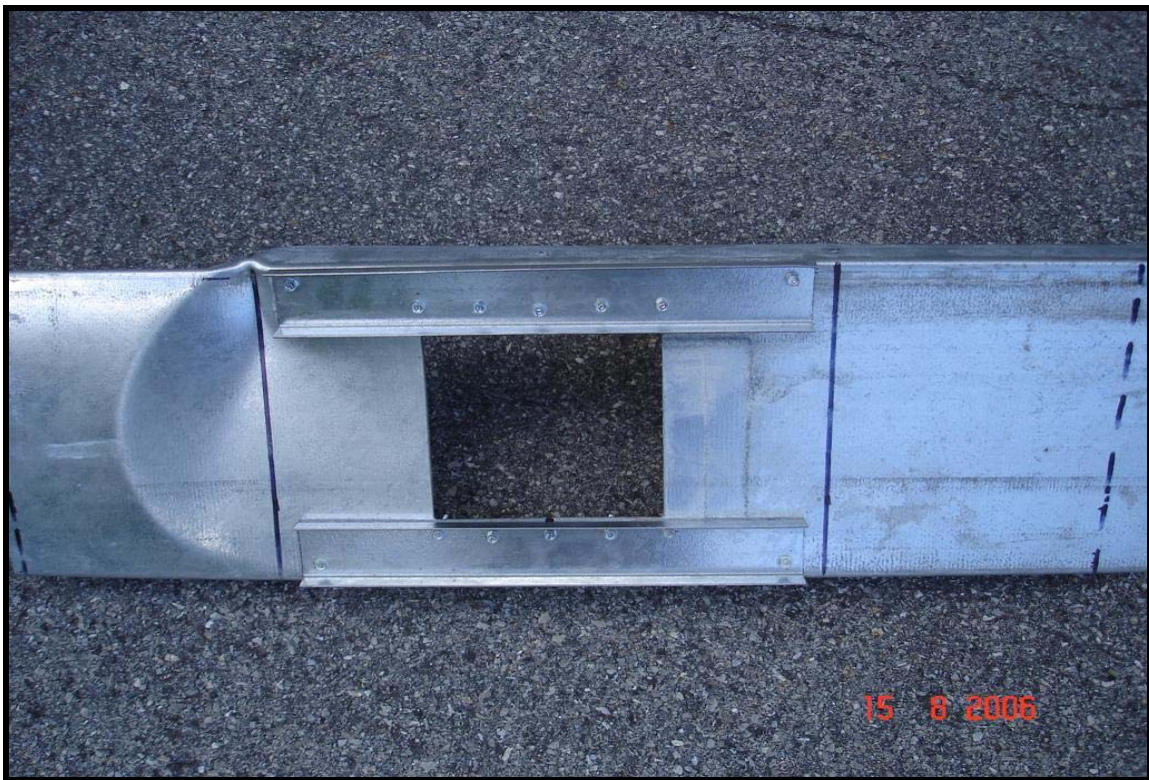
Figure B.3.6 Typical flexural failure for specimens having reinforced (Scheme-“C”) square web opening
