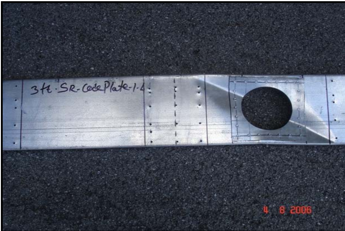
Figure C.2.2 Typical failure for specimens having reinforced (Scheme-“A”) circular web openings
