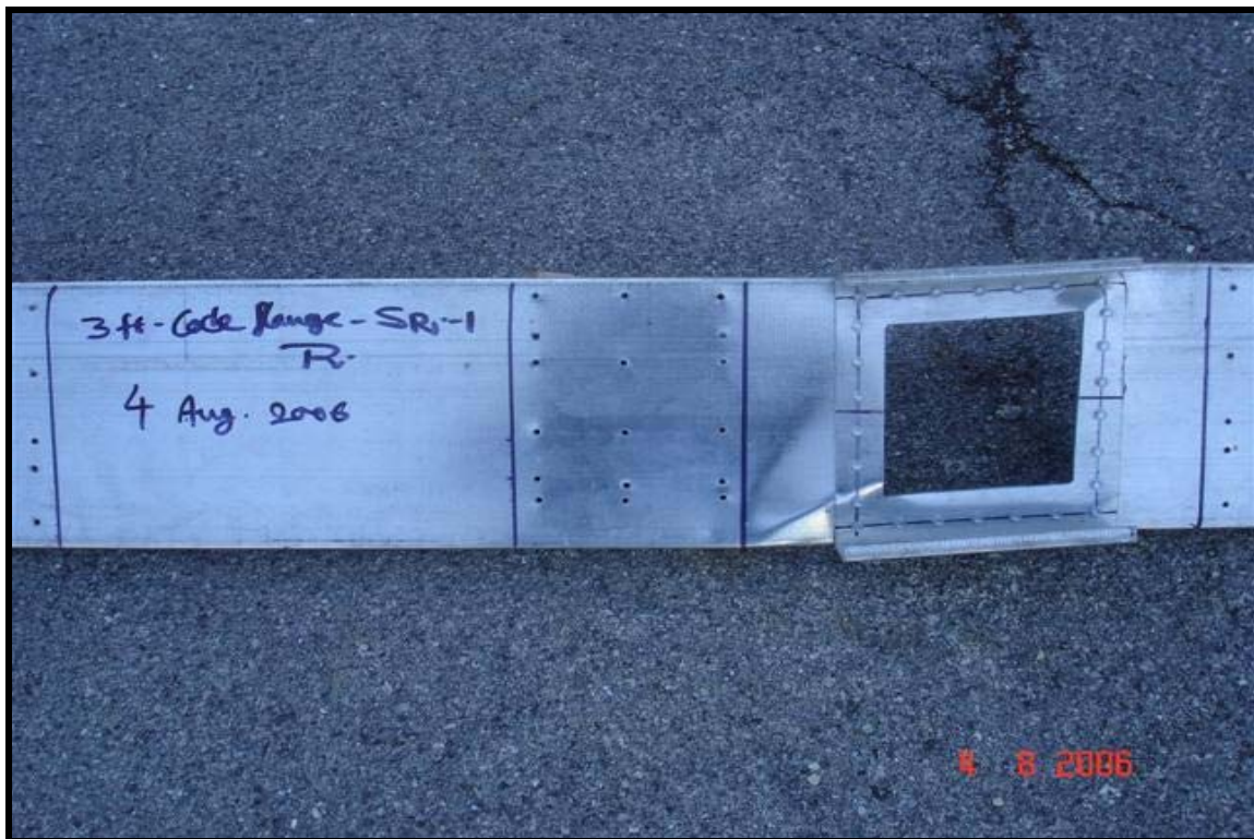
Figure C.3.4 Typical failure for specimens having reinforced (Scheme-“B”) square web openings
