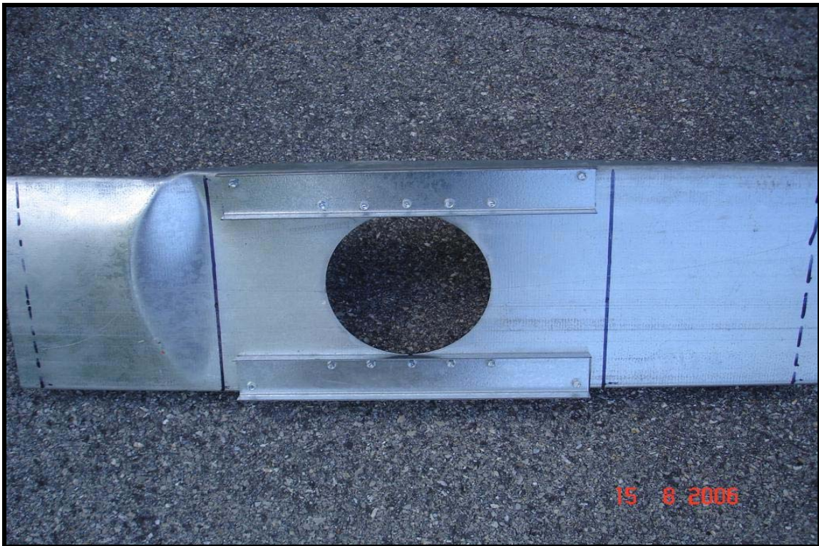
Figure B.2.6 Typical flexural failure for specimens having reinforced (Scheme-“C”) circular web openings
