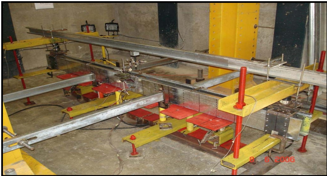
Figure 2.2 Photograph of the Flexural Test Setup
