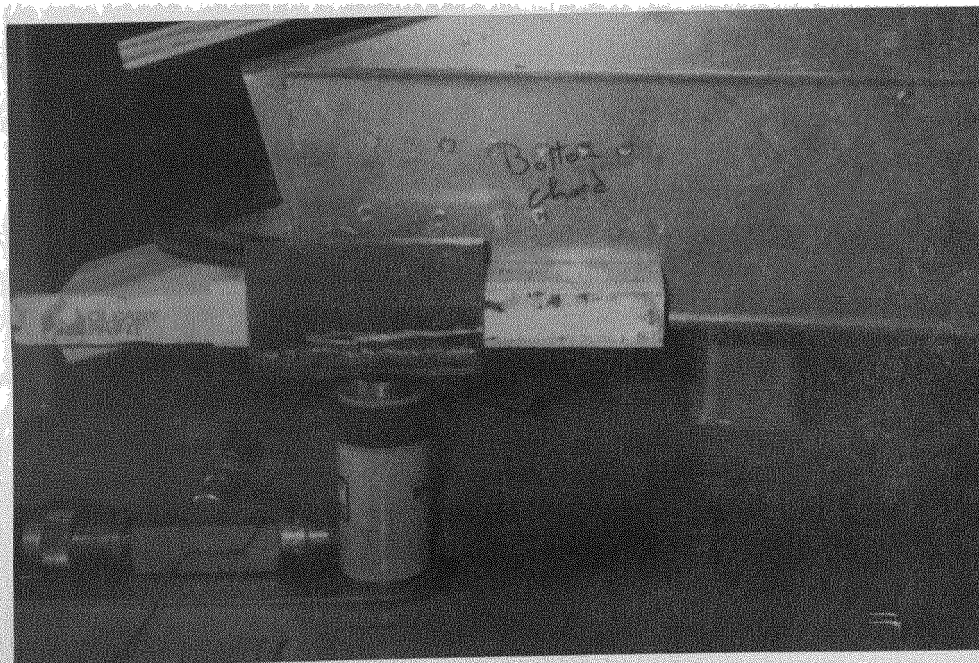
Figure 7. End of Truss Assembly Resting on Load Cell
