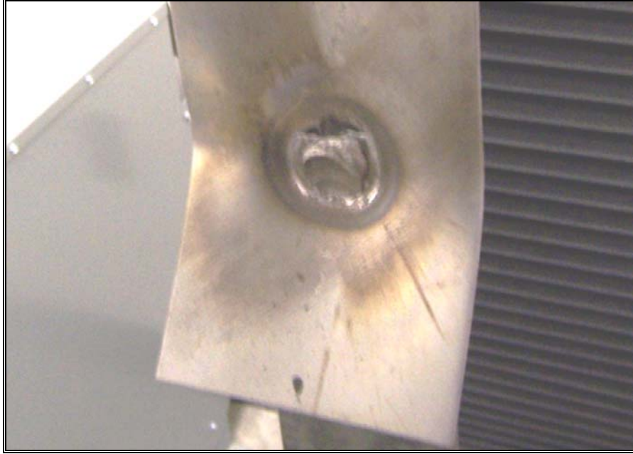
Figure 3-5: Sheet Tear Failure
