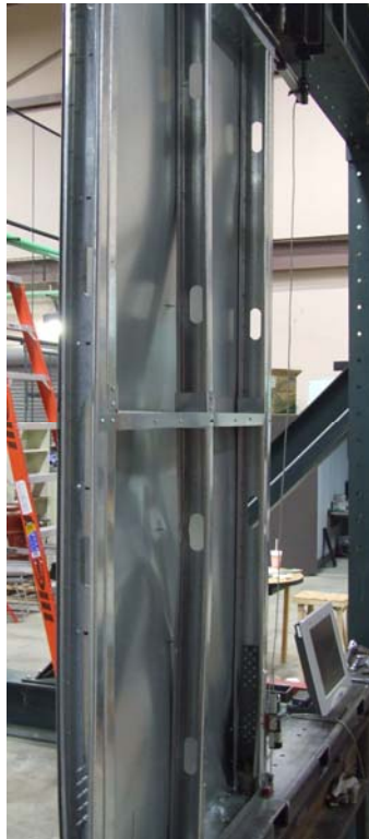
Figure 25 Failure mode of test 8×4×350-43×33-2-C1-C
