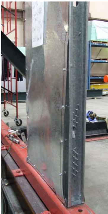
Figure 14 Screw pull-out failure on 27-mil sheet steel shear wall
