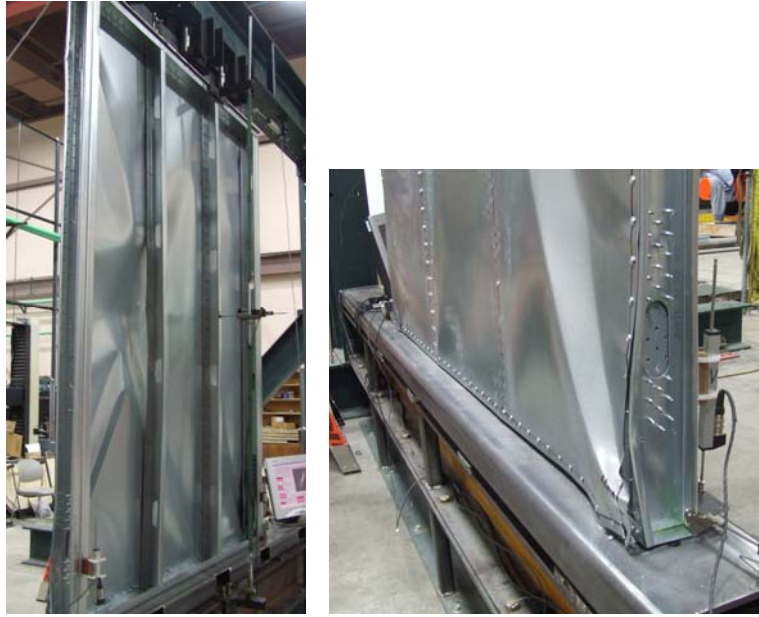
Figure 23 Failure mode of test 8x6x350-54x33-2-C1-B
