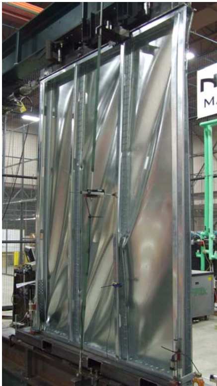
Figure 28 Failure mode of 8x6x350-43x27-2-M1-D
