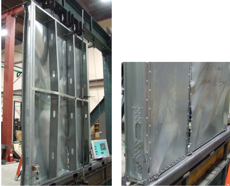
Figure 22 Failure mode of test 8x6x600-43x30-2-C1-C
