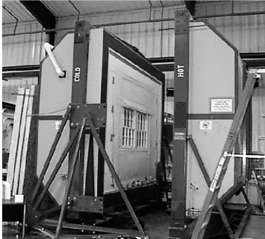
Figure 6 - Rotatable Guarded Hot Box
