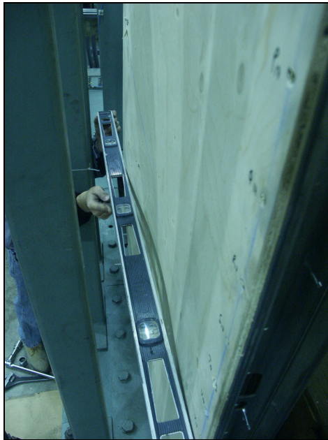
Figure 2.20: Shear Buckling of Sheathing
